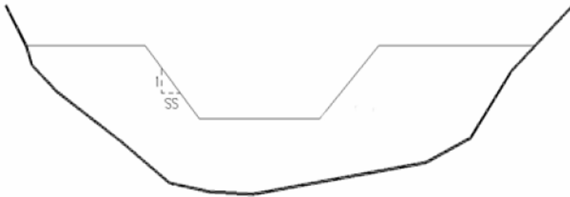
Figure 2.4. Explanation of the breach side slope. Presented as 1/SS in Chapter 2.3.1-2.3.4.
