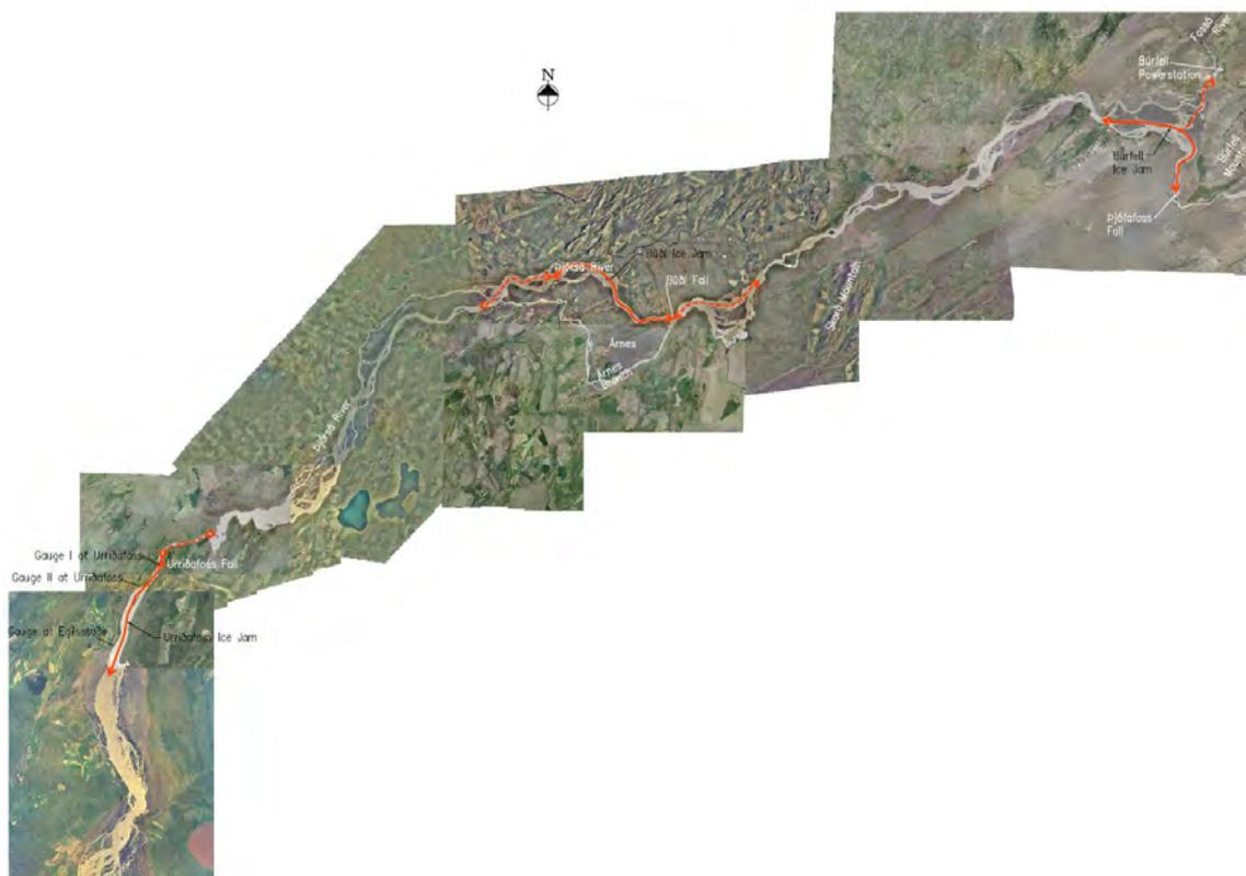
**Figure 3.1** Overview of Lower Þjórsá River. Gauging stations are marked in and the location of the ice jams that formed regularly before the ice got trapped in the upper reaches due to reservoirs and other constructions. An A3 version of this figure can be found at the end of this report before the Appendixes.
