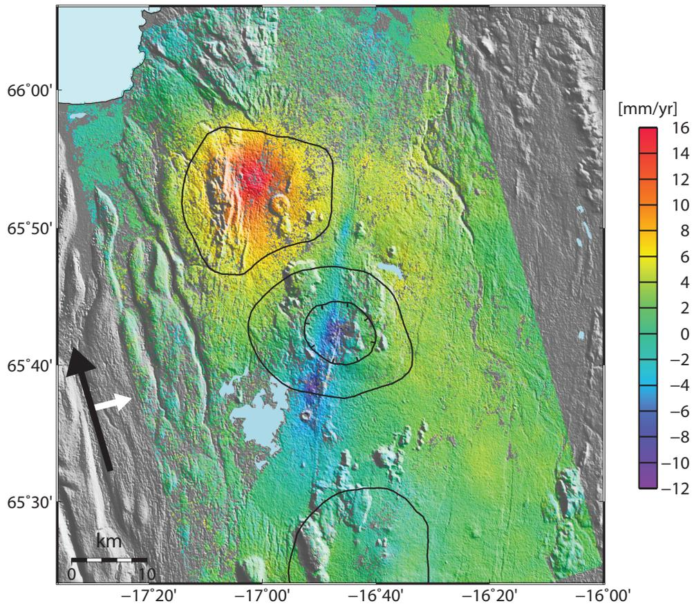
Figure 4.3: Average LOS velocity estimate for ascending Envisat track 230, spanning the period 2003-2008. The black arrow shows the flight direction, while the white arrow shows the projection of the look direction on the horizontal plane.
