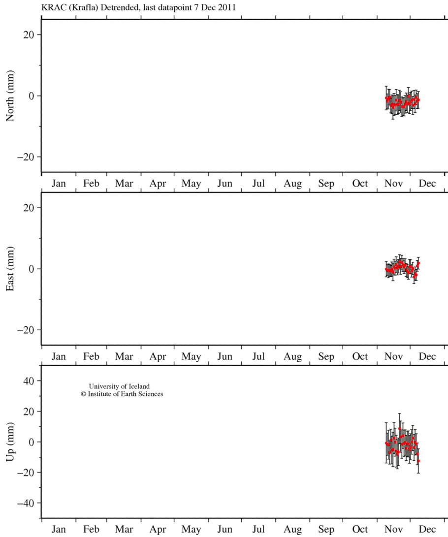
Figure 3.5: Time series plot showing deformation of station KRAC in north, east and up components. Data collection started on November 8th 2011, the graph was extracted on December 7th 2011.
