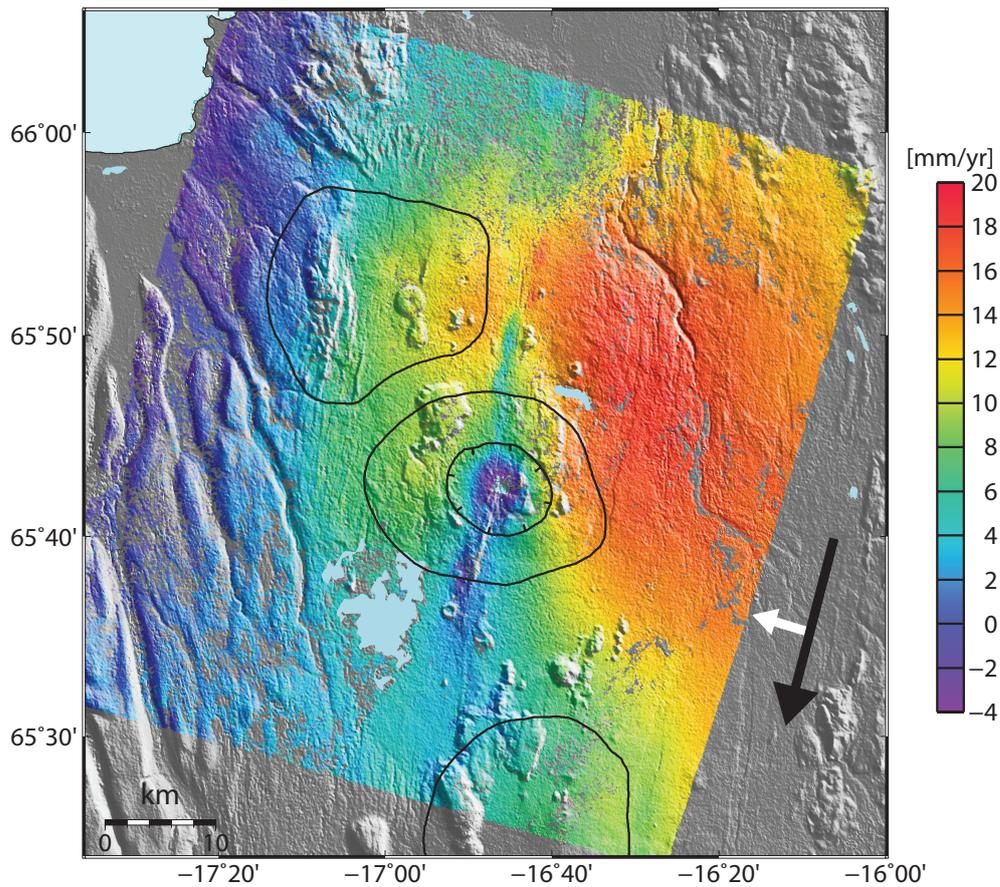
Figure 4.1: Average LOS velocity estimate for descending ERS track 9, spanning the period 1993-2002. The black arrow shows the flight direction, while the white arrow shows the projection of the look direction on the horizontal plane.
