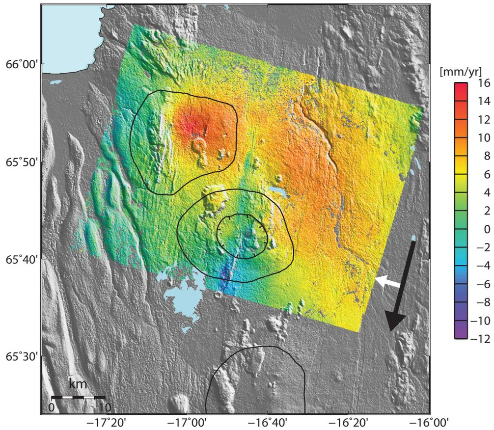
Figure 4.2: Average LOS velocity estimate for descending Envisat track 9, spanning the period 2003-2010. The black arrow shows the flight direction, while the white arrow shows the projection of the look direction on the horizontal plane.
