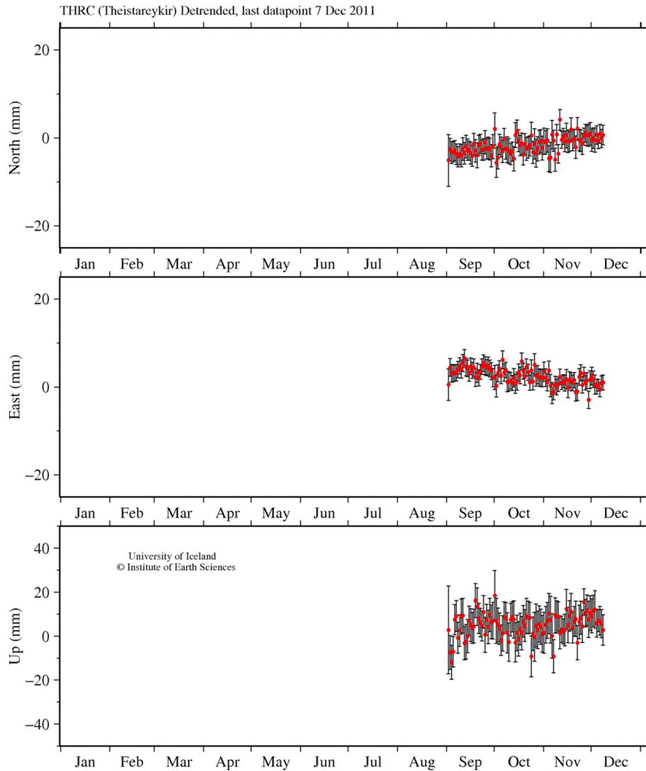
Figure 3.4: Time series plot showing deformation of station THRC in north, east and up components. Data collection started on September 1st 2011, the graph was extracted on December 7th 2011.
