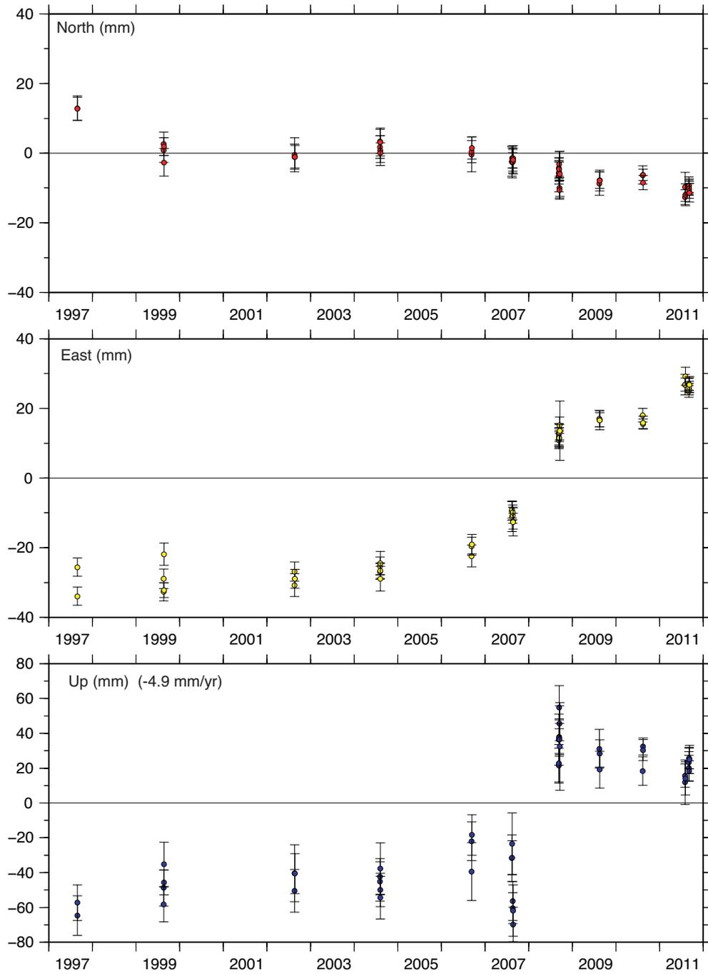
Figure 2.3: Detrended time series results in north, east and up components of station THER between 1997 and 2011.
