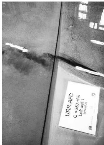
Figure 3.7: Photograph of a dye test from preliminary tests in the physical model showing diversion of flow away from left approach bank.
