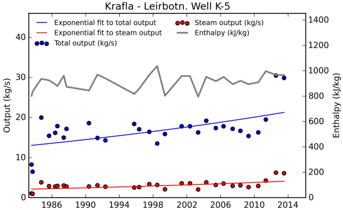
Figure A 7. Enthalpy, output and steam decay in well K-5.
