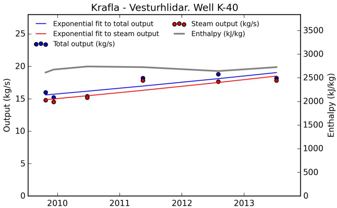
Figure A 26. Enthalpy, output and steam decay in well K-40.
