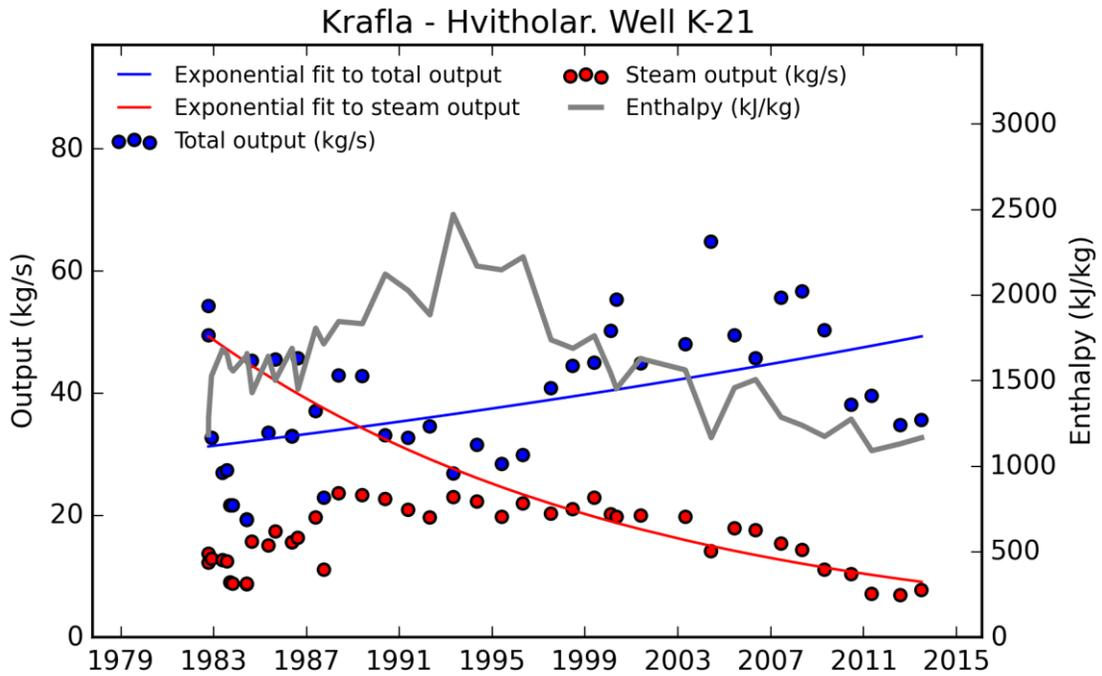
Figure A 16. Enthalpy, output and steam decay in well K-21.
