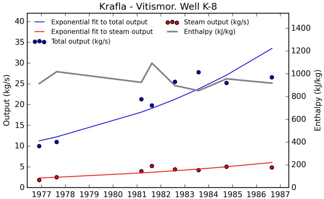
Figure A 8. Enthalpy, output and steam decay in well K-8.
