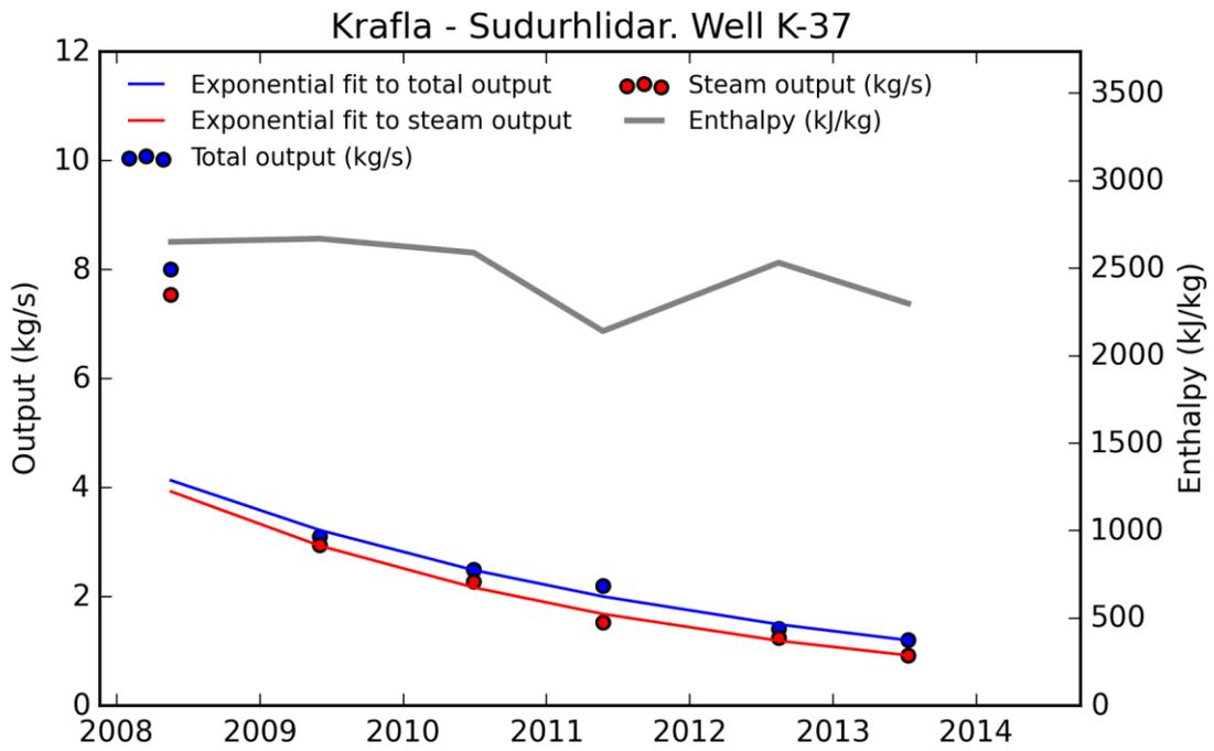
Figure A 25. Enthalpy, output and steam decay in well K-37.
