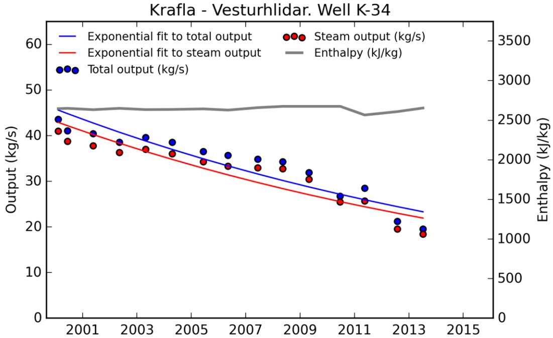
Figure A 23. Enthalpy, output and steam decay in well K-34.
