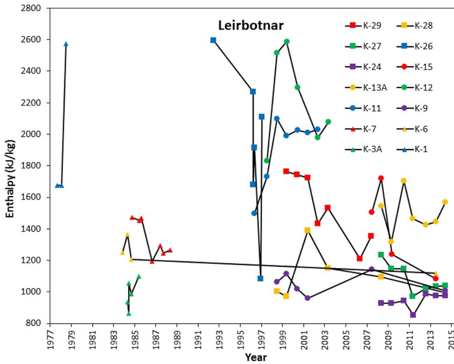
Figure A 5. Enthalpy vs. time of each well included in this study in Leirbotnar.
