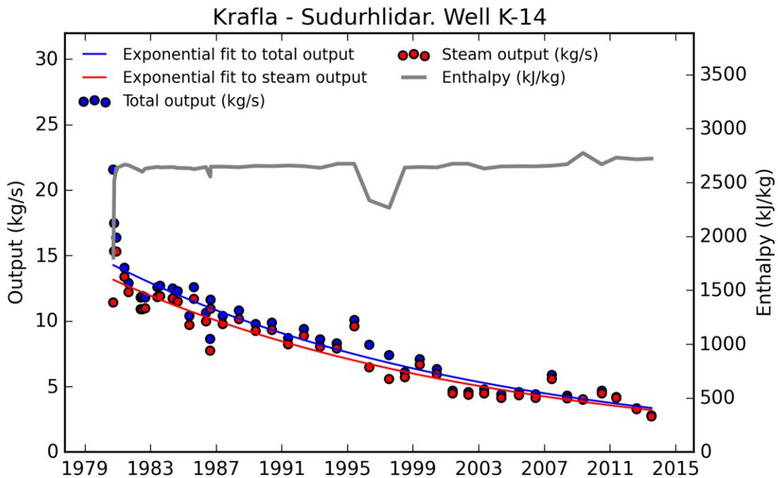
Figure A 10. Enthalpy, output and steam decay in well K-14.
