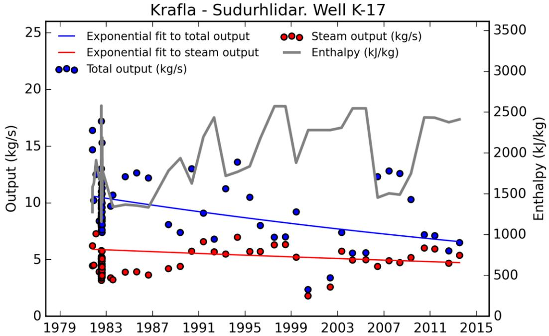
Figure A 13. Enthalpy, output and steam decay in well K-17.
