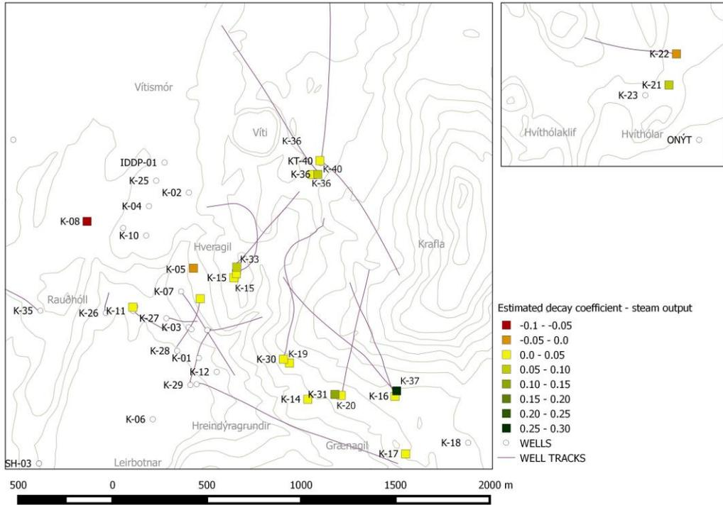
**Figure 53.** The estimated steam output decay in % per year for 20 wells in the Krafla caldera. Red indicates increased steam output, the orange colored data points indicate that no decay took place in the well, while yellow and green refer to decreased steam output from wells.
