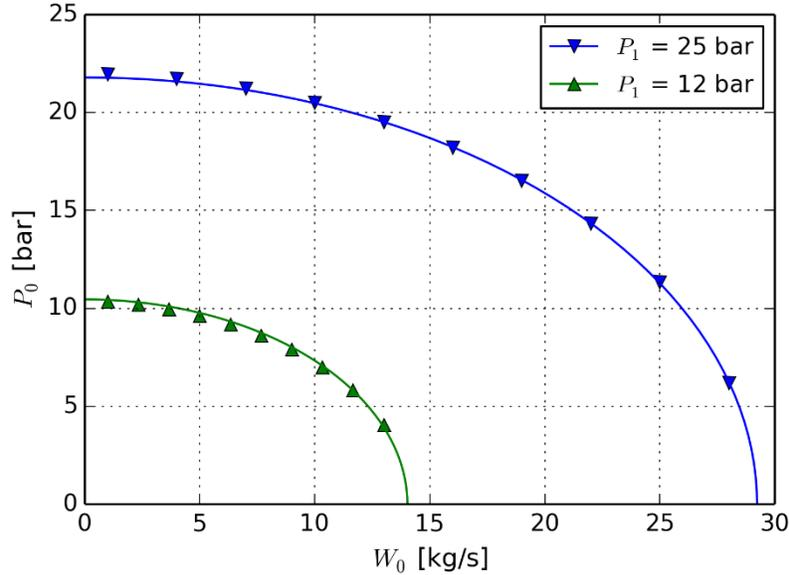
**Figure 57.** The well-head pressures calculated by WellSim are fitted at constant enthalpy to find  $a_0$  and  $b_0$  for a given enthalpy.
