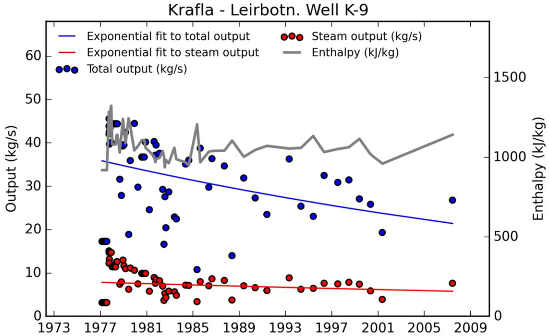
Figure A 9. Enthalpy, output and steam decay in well K-9.
