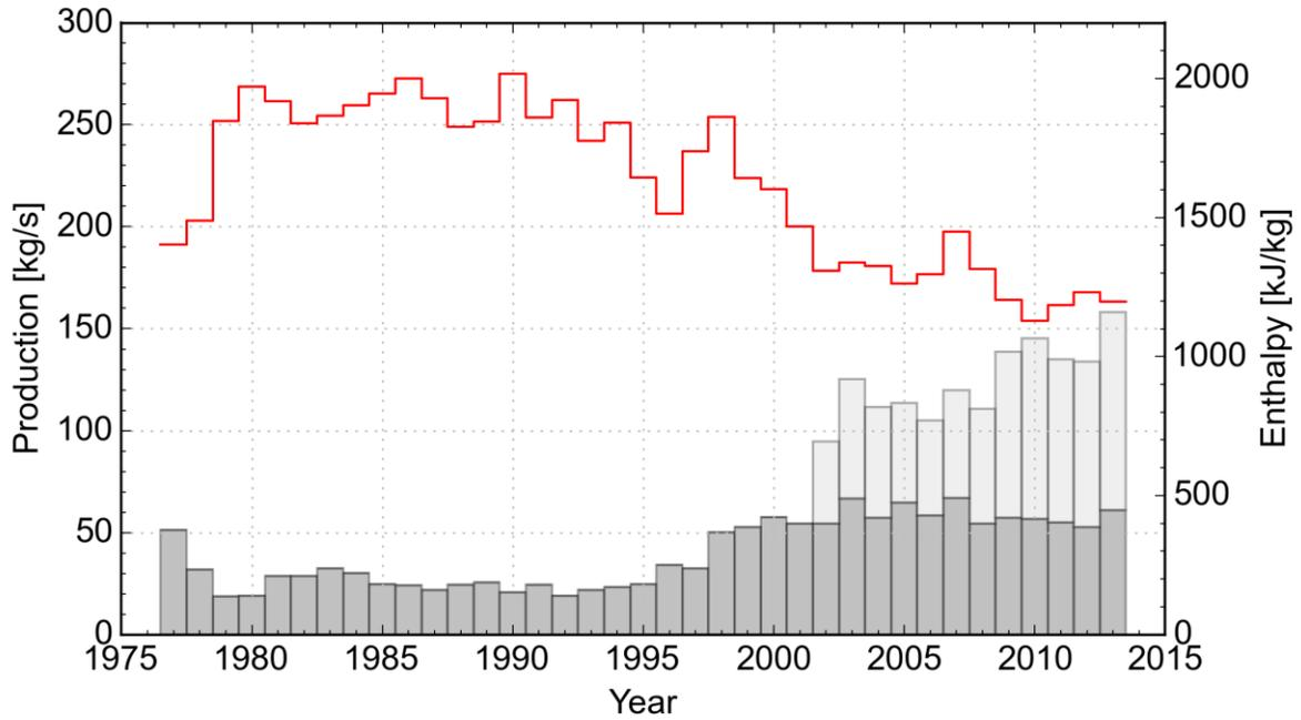
**Figure 44.** *Leirbotnar lower system (9 wells out of which 3 are currently producing wells) average mass production per year (columns) and weighted yearly mean enthalpy (red line).*
