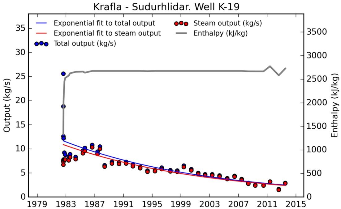
Figure A 14. Enthalpy, output and steam decay in well K-19.
