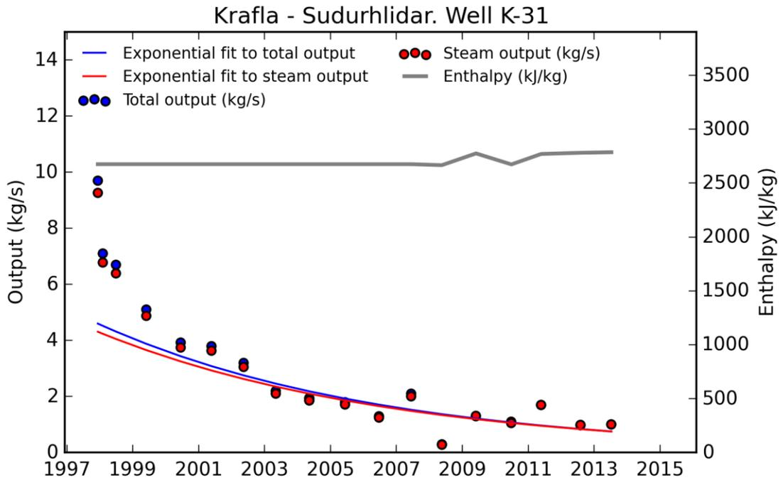
Figure A 20. Enthalpy, output and steam decay in well K-31.
