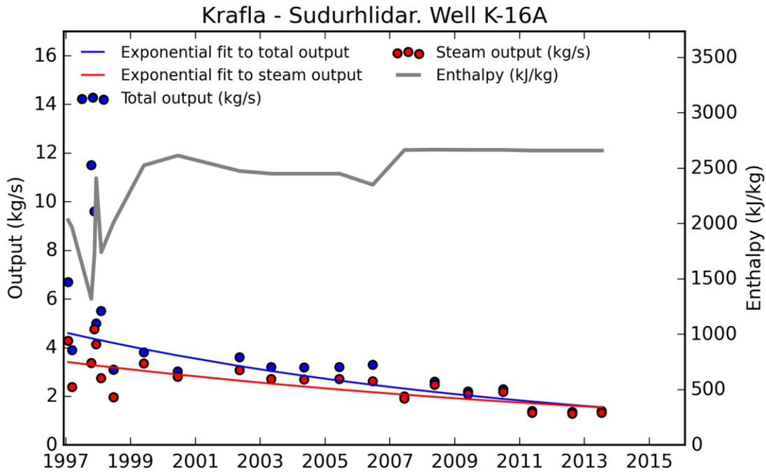
Figure A 12. Enthalpy, output and steam decay in well K-16A.
