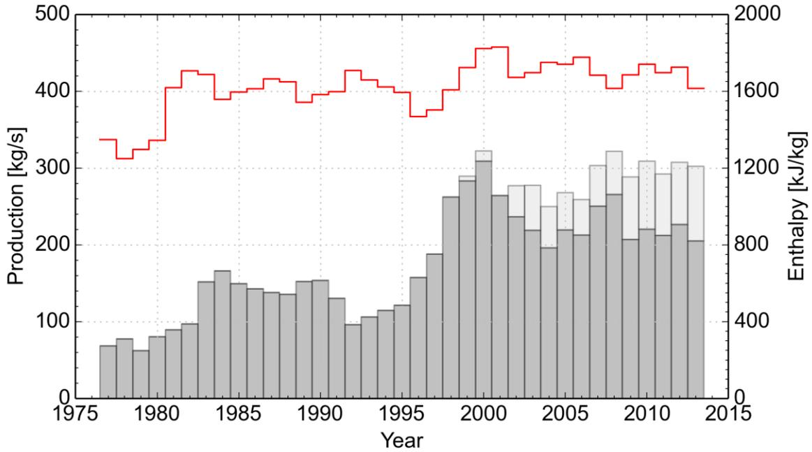
**Figure 42.** Average total mass production per year (columns) and weighted yearly mean enthalpy (red line) for all Krafla production wells. The darker shaded bars represent production while the lighter shaded bars represent reinjection.
