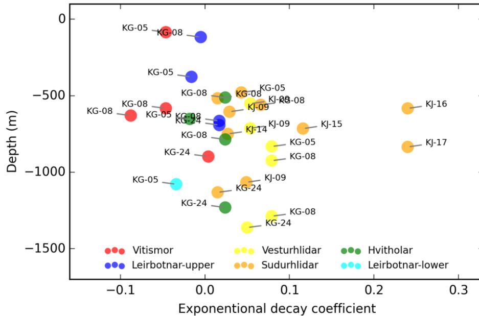
**Figure 52.** Total output decay plotted against feed zone depth in the wells analyzed in this section. The points in the plot have been color coded according to the sub-fields of Krafla to give an idea of how decay and feed zone depth vary between areas. Negative decay implies an increase in output.
