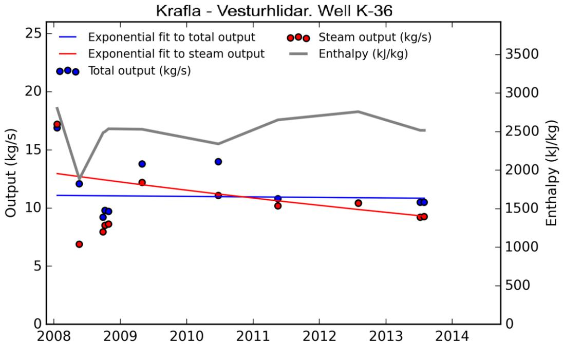
Figure A 24. Enthalpy, output and steam decay in well K-36.
