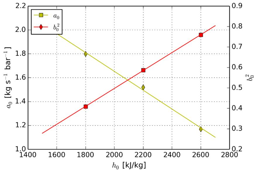
**Figure 58.** Regression analysis of  $a_0$  and  $b_0^2$  versus enthalpy used to determine  $\alpha_0$ ,  $\beta_0$ ,  $\gamma_0$  and  $\delta_0$  for well K-31.
