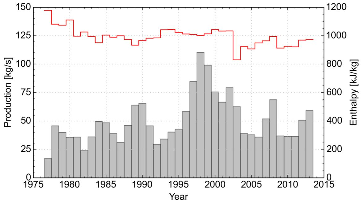
**Figure 45.** *Leirbotnar upper system (5 production wells, 2 currently producing wells) average mass production per year (bars) and weighted yearly mean enthalpy (red line).*
