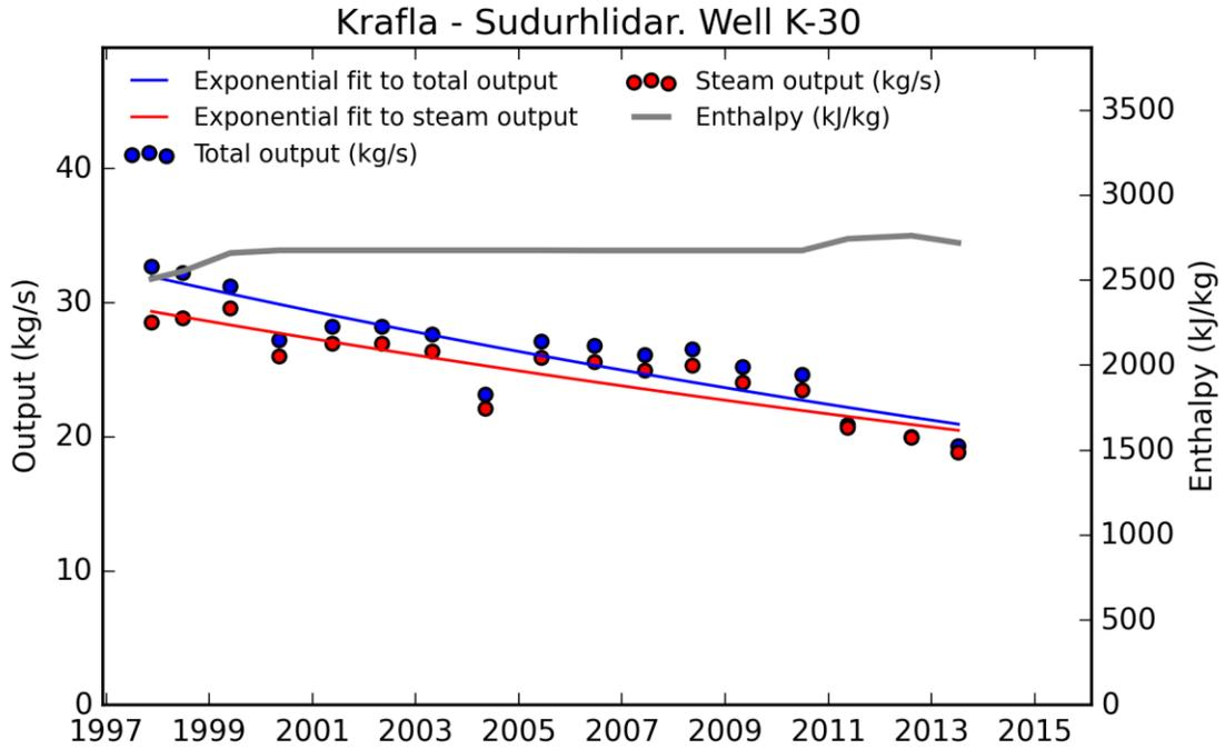
Figure A 19. Enthalpy, output and steam decay in well K-30.
