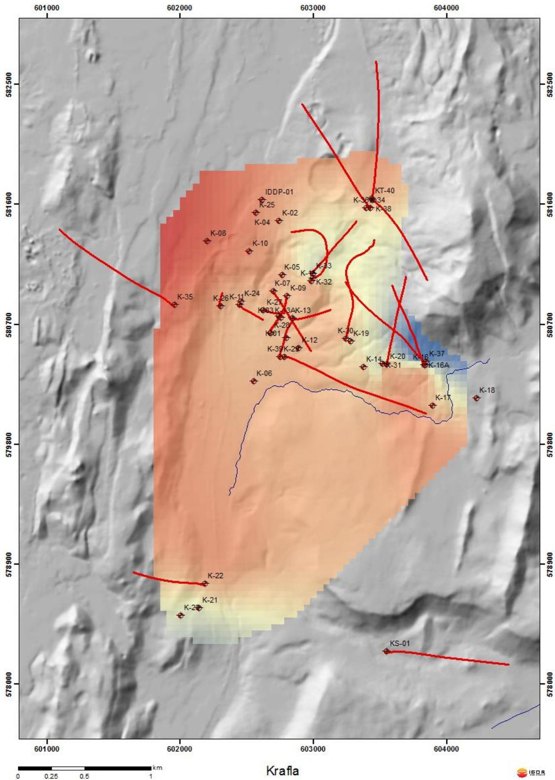
**Figure 56.** Steam decay of selected wells mapped onto the surface of the Krafla geothermal field. Cold colors indicate decay while hot colors indicate increased output.
