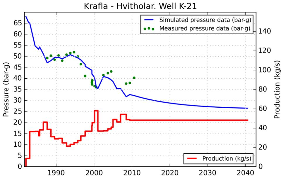
**Figure 50.** Pressure and production data for Hvíthólar, the fit to the pressure data from well K-21 is obtained using lumped parameter modeling, including a 30-year forecast.
