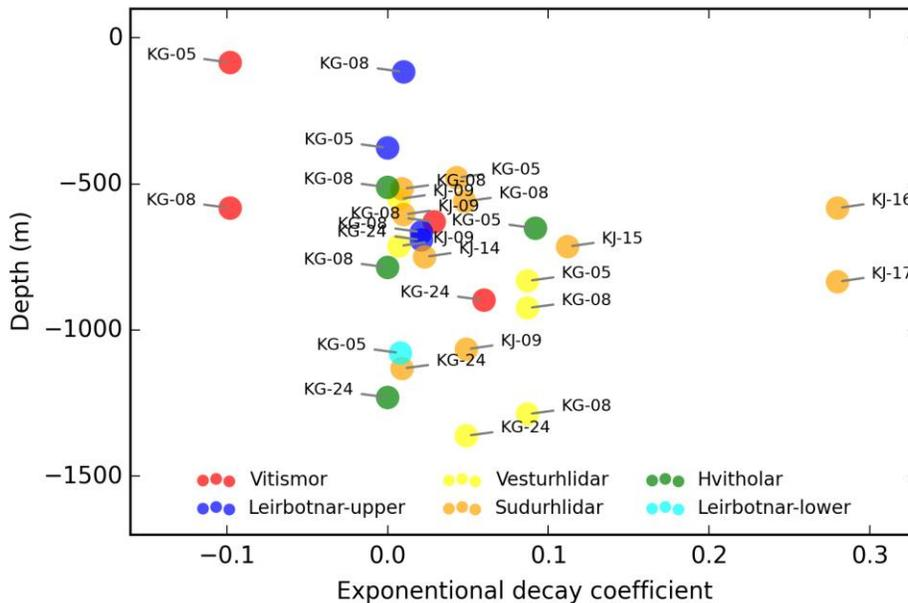
**Figure 54.** Steam output decay plotted against feed zone depth in the wells analyzed in this section. The feed zone depths are not steam feed zones and do not reflect the origin of steam specifically. The points in the plot have been color coded according to the sub-fields of Krafla to give an idea of how decay and feed zone depth vary between areas.
