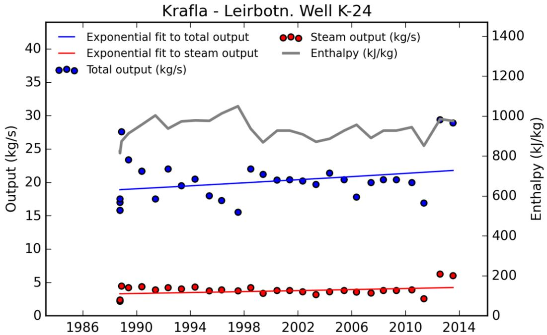
Figure A 18. Enthalpy, output and steam decay in well K-24.
