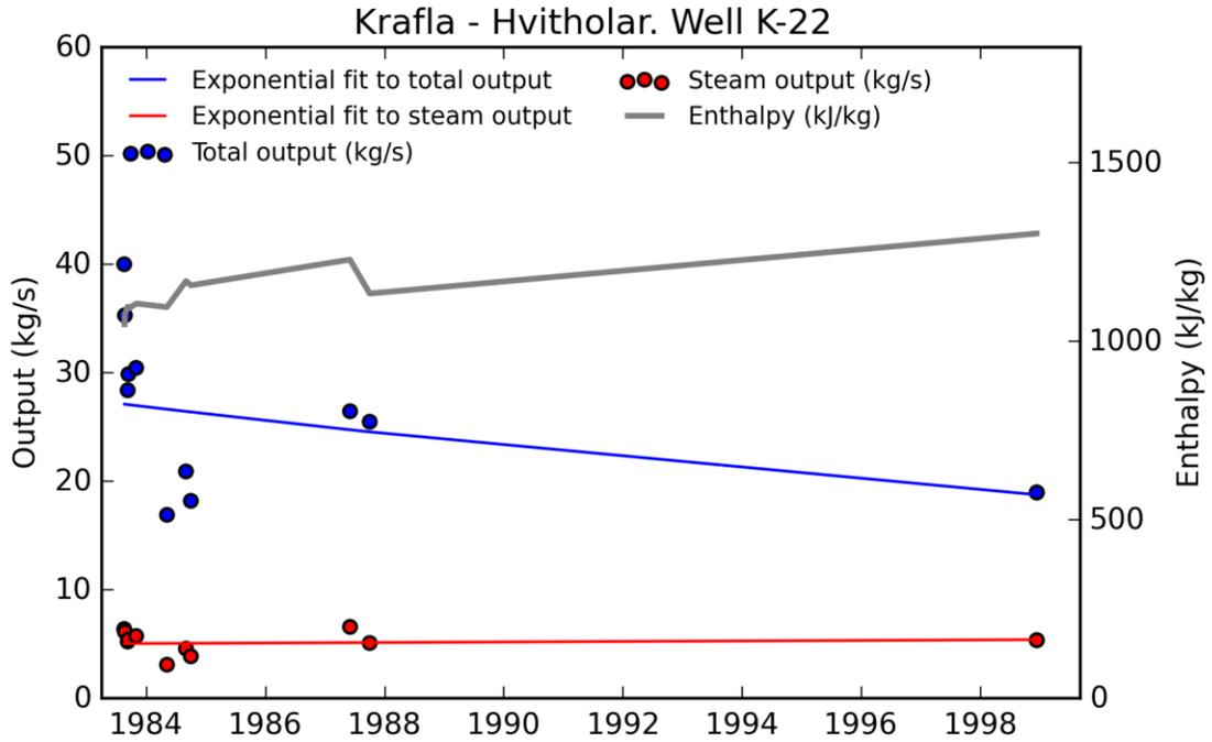
Figure A 17. Enthalpy, output and steam decay in well K-22.
