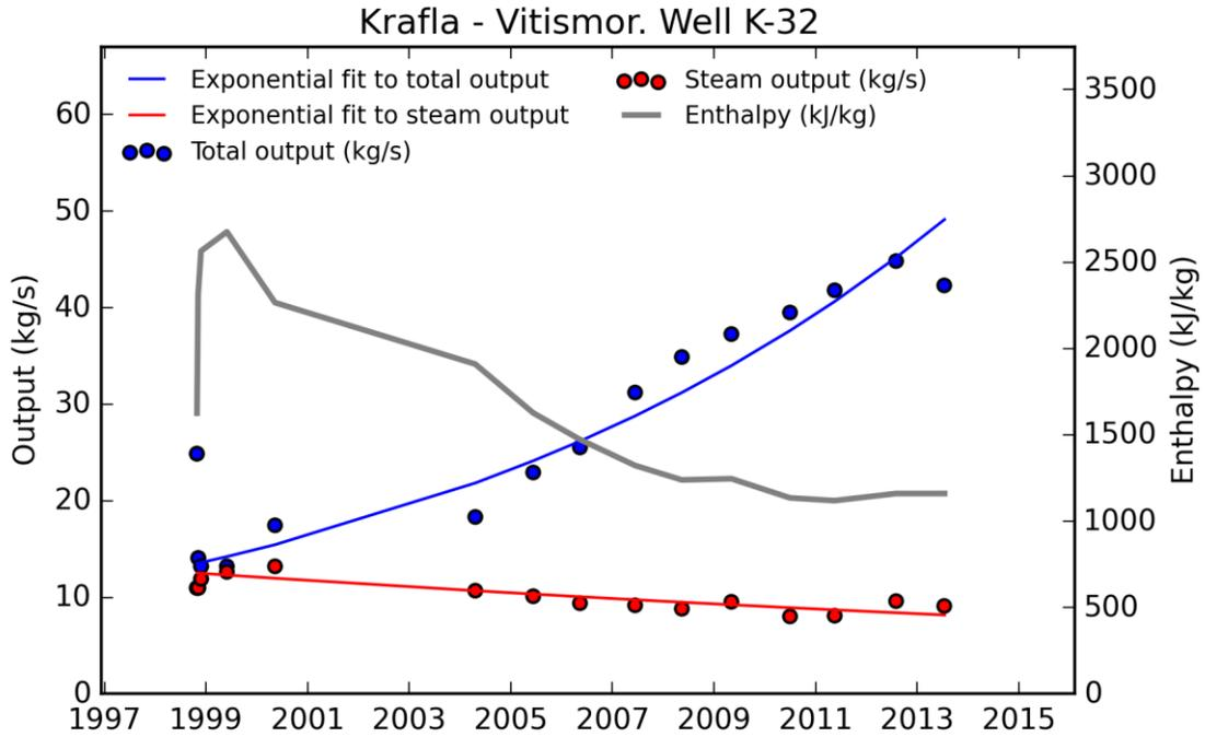
Figure A 21. Enthalpy, output and steam decay in well K-32.
