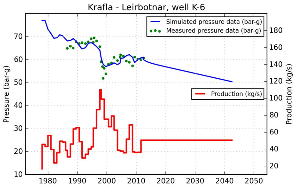
**Figure 49.** Pressure and production data for Leirbotnar; the fit to the pressure data for well K-6 is obtained using lumped parameter modeling, including a 30 year forecast.
