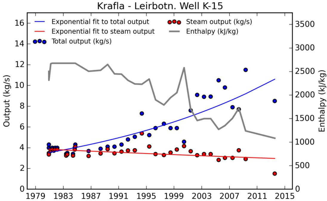
Figure A 11. Enthalpy, output and steam decay in well K-15.
