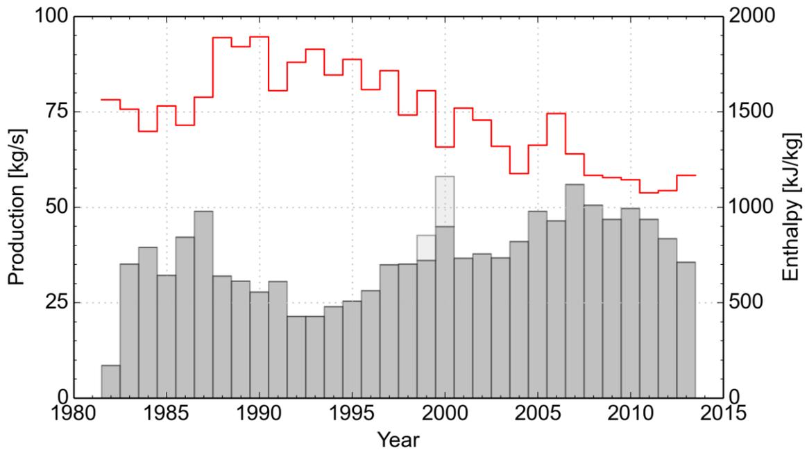
**Figure 43.** Hvíthólar (well K-21) average mass production per year (bars) and weighted yearly mean enthalpy (red line). The darker shaded bars represent production while the lighter shaded bars represent reinjection.
