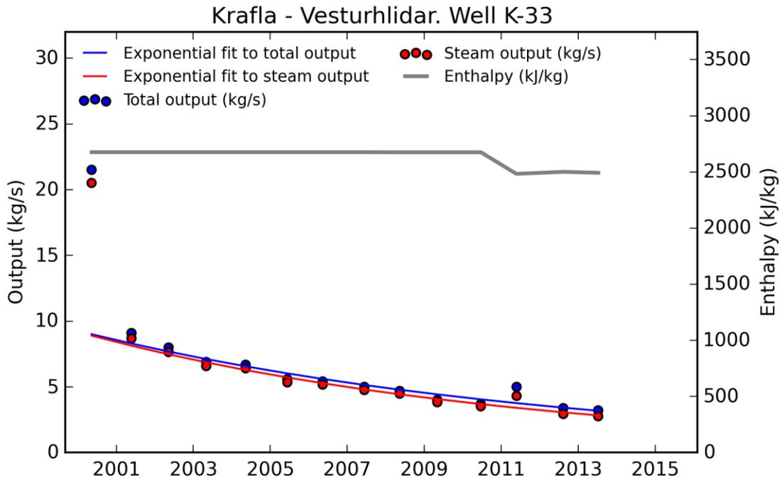
Figure A 22. Enthalpy, output and steam decay in well K-33.
