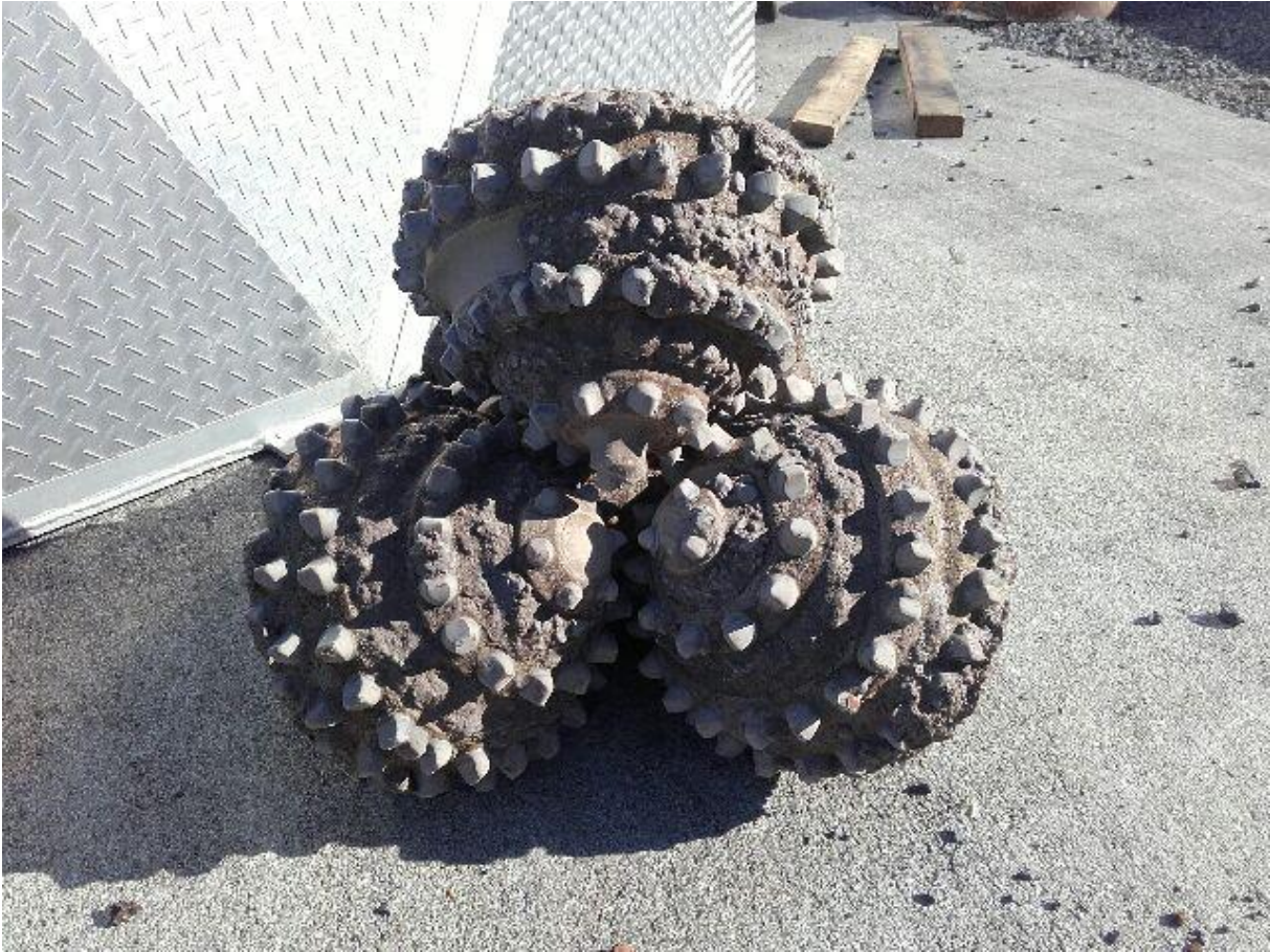
Figure 8. The 21" drill bit, after the pre-drilling.
