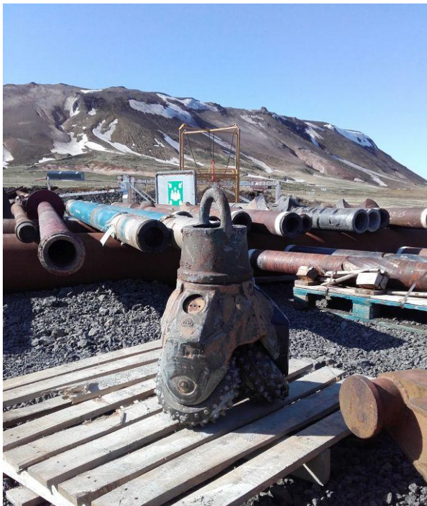
Figure 9. The 17½" bit that was used for drilling for the 13 5/8" anchor casing, Mt. Bæjarfjall in the background.
