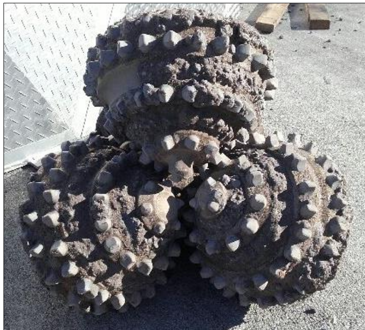
Figure 6. The 21" drill bit, after pre-drilling of PG-11.
