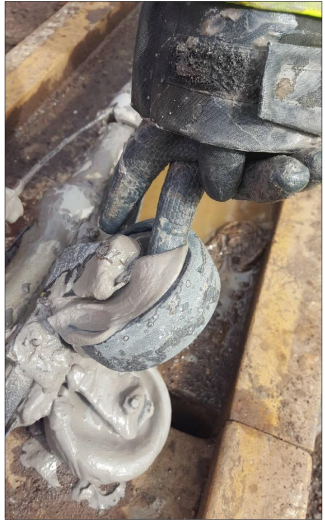
Figure 4. Logging engineers preparing to run the CBL tool into the well (left) and the centralizer caked in mud on return from the logging of well K41.
