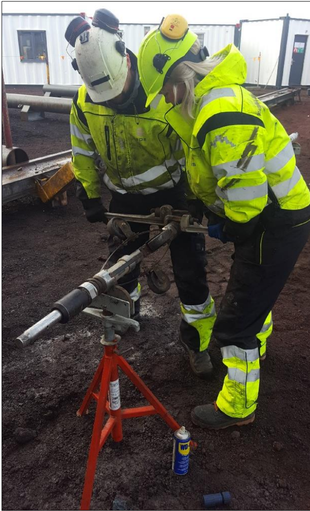
Figure 4. Logging engineers preparing to run the CBL tool into the well (left) and the centralizer caked in mud on return from the logging of well K41.
