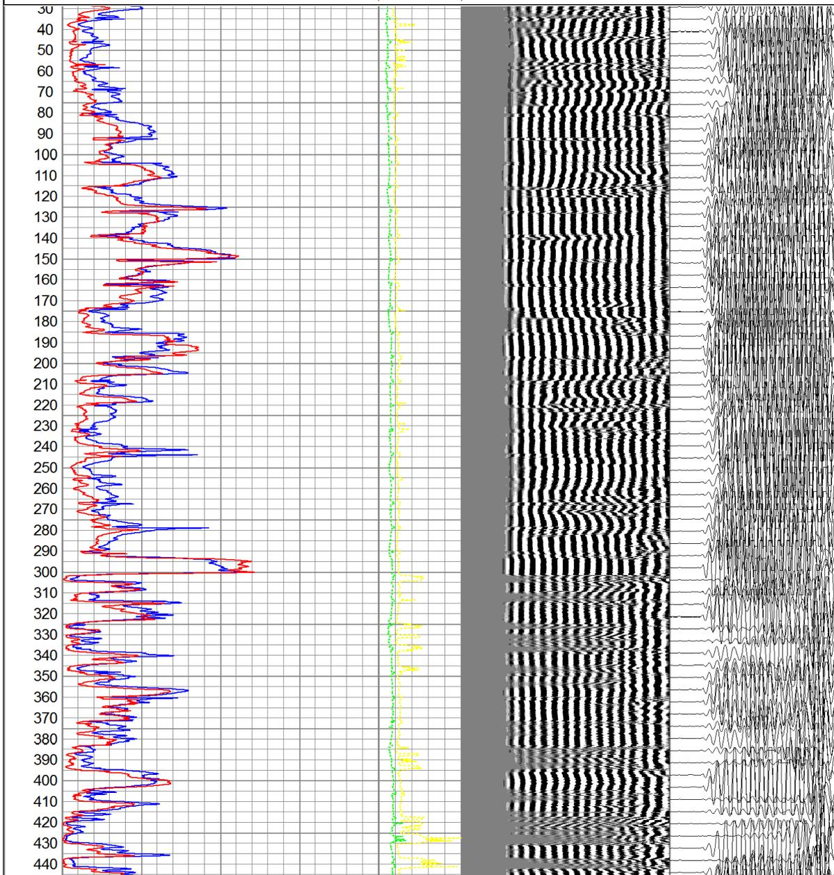
Figure 17. Cement Bond Log – Production casing, ~18 hours after cementing.
