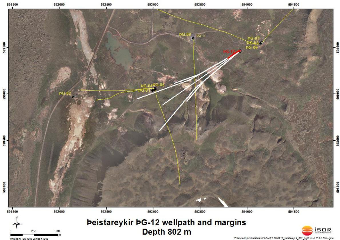
**Figure 1.** Aerial photograph of Peistareykir. Location of current drillpads and production wells and their trace in the Peistareykir geothermal field. The red line represents the trace of well ÞG-12 to 806.0 m depth (end of phase 2).
