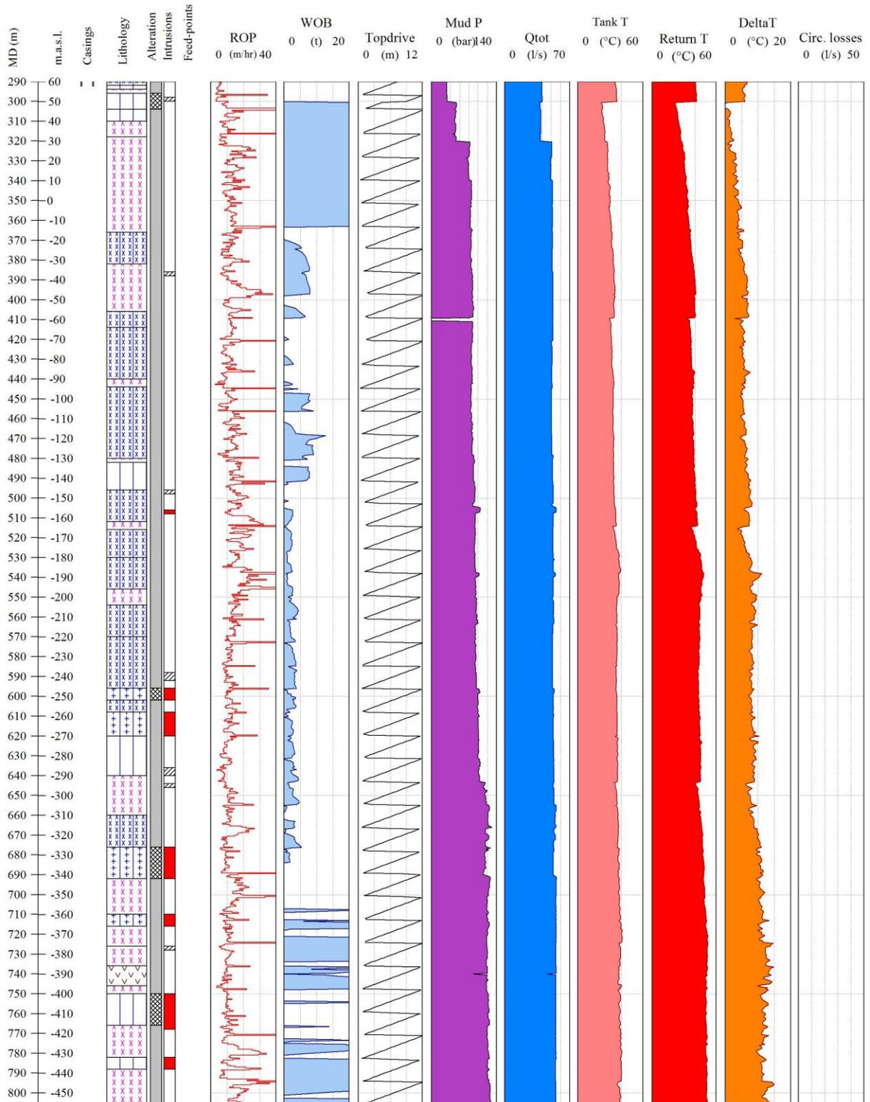
Figure 9. Lithology and drilling data in well ÞG-12 from 290 to 806 m.
