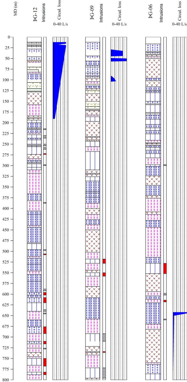
**Figure 1.** Lithology logs and loss circulation zones from 0 to 800m for wells ÞG-12, ÞG-09 and ÞG-06
