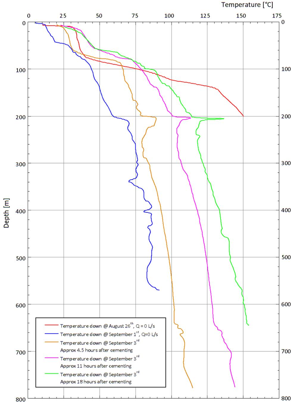
**Figure 14.** Temperature log compilation for phase 2 of well ÞG-12.
