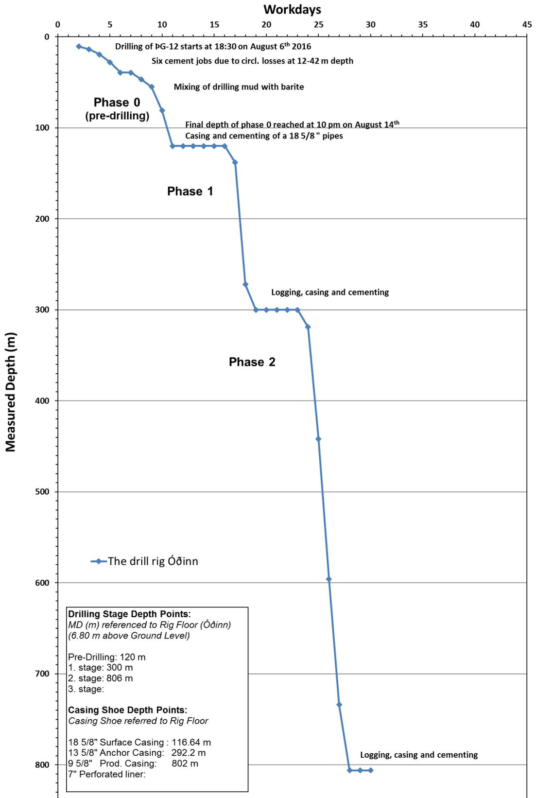
Figure 1. Drilling progress of PG-12 until present.
