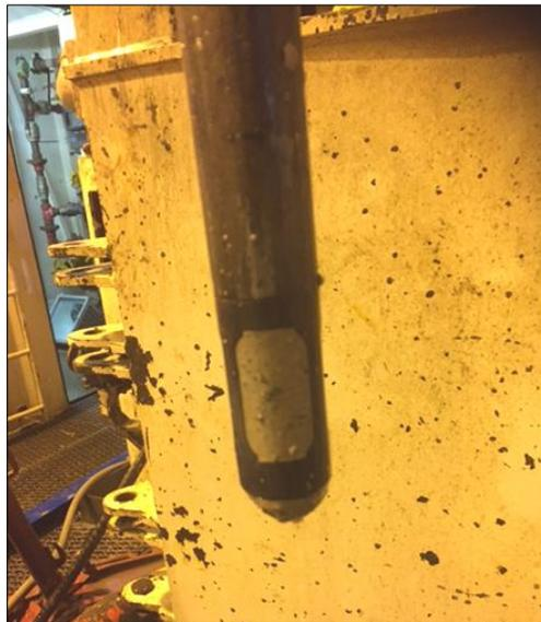
**Figure 13.** *The temperature logging tool at surface after logging September 1<sup>st</sup> with the heat sensor covered by mud.*
