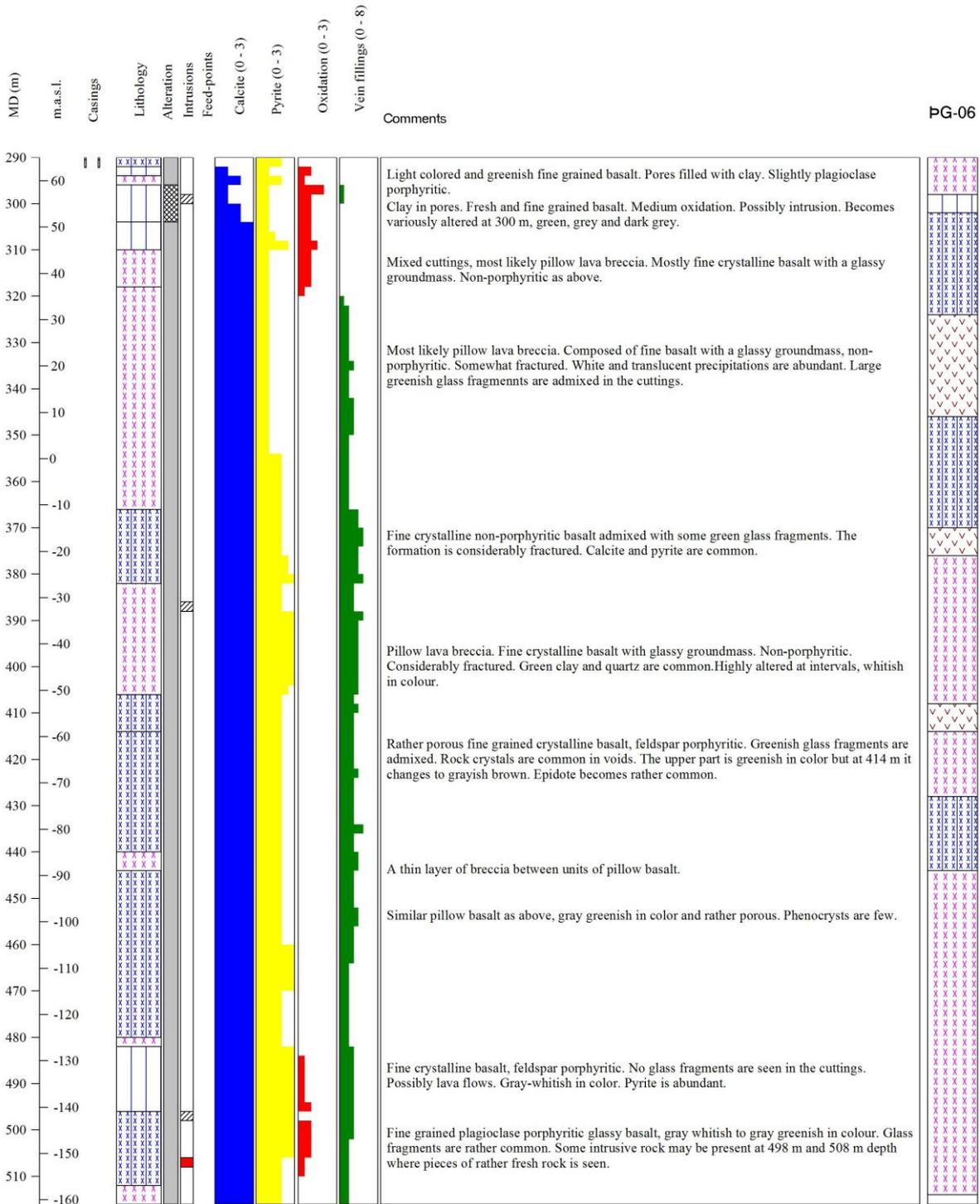
Figure 1. Lithology column from ÞG-12 from 290-516 m depth. Well ÞG-06 is shown for comparison.
