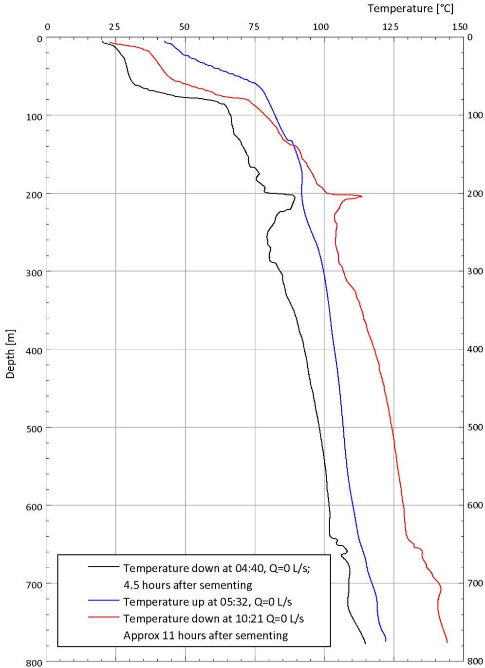
**Figure 3.** Temperature logs run after cementing of production casing (before and after CBL log)
