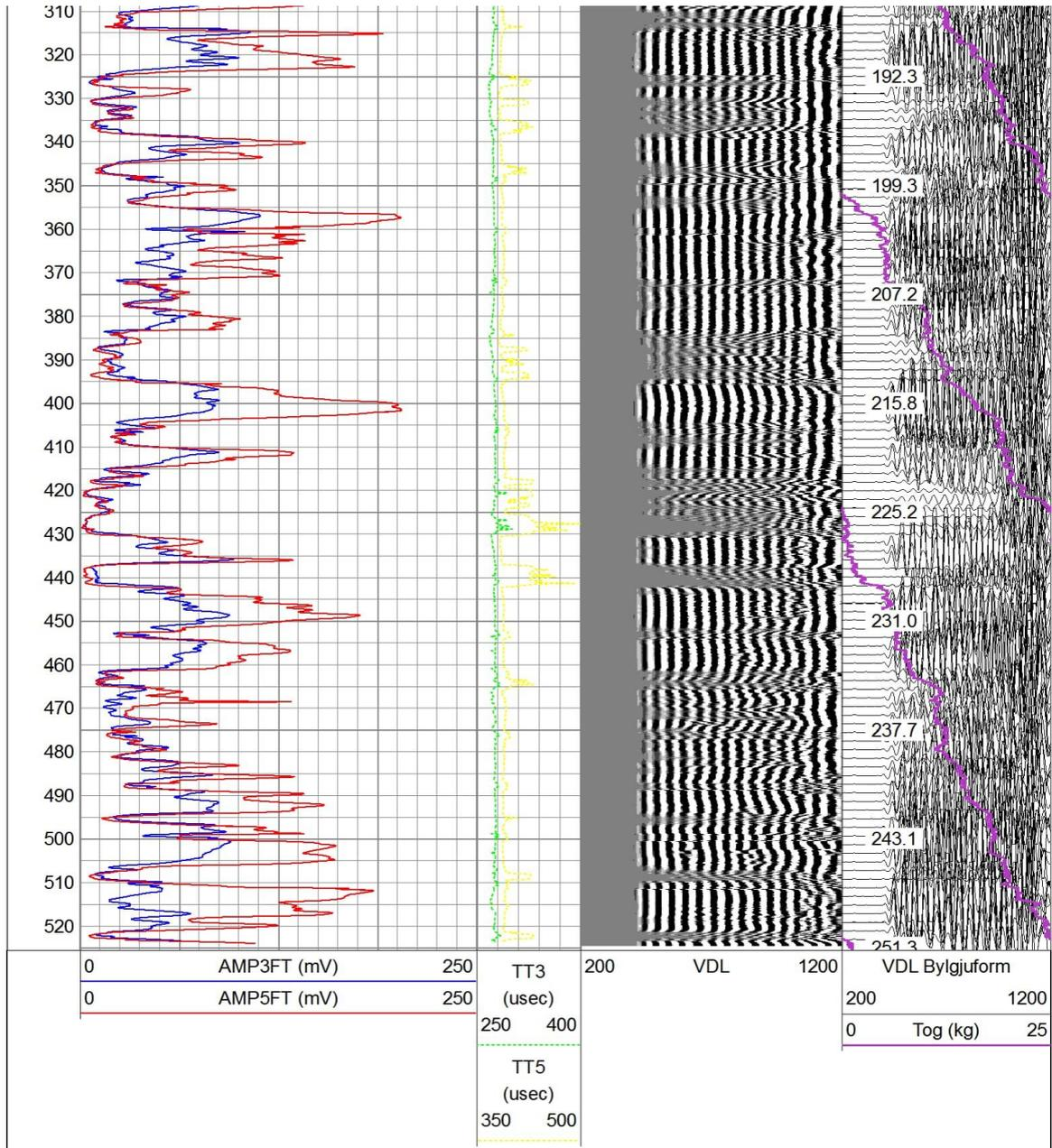
**Figure 2.** Low res. CBL log run about 18hours after cementing of production casing
