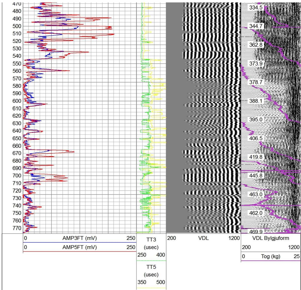
**Figure 4.** Low res. CBL log run about 9hours after cementing of production casing
