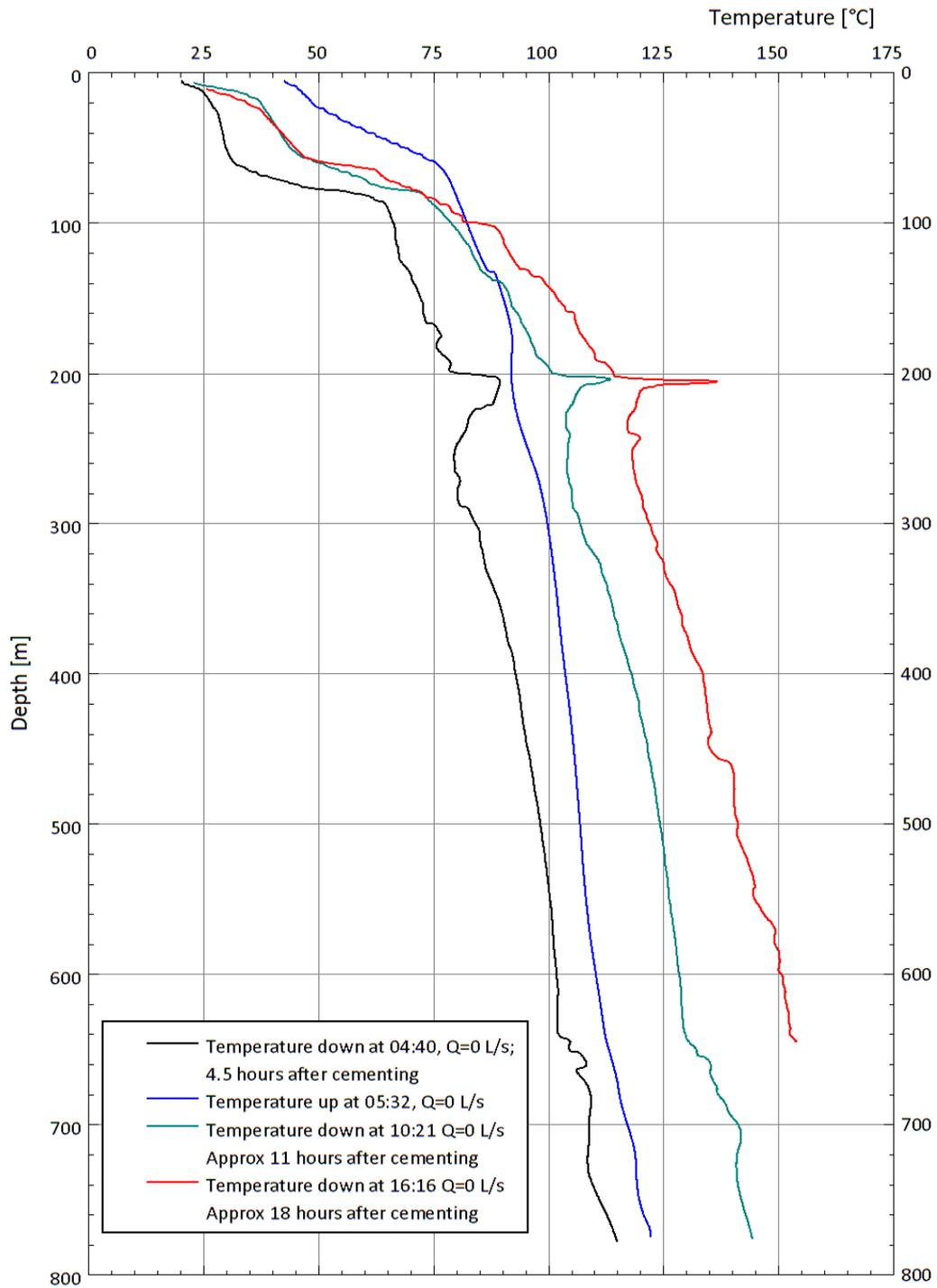
**Figure 1.** Compiled temperature logs run in the 9 5/8" production casing after cementing
