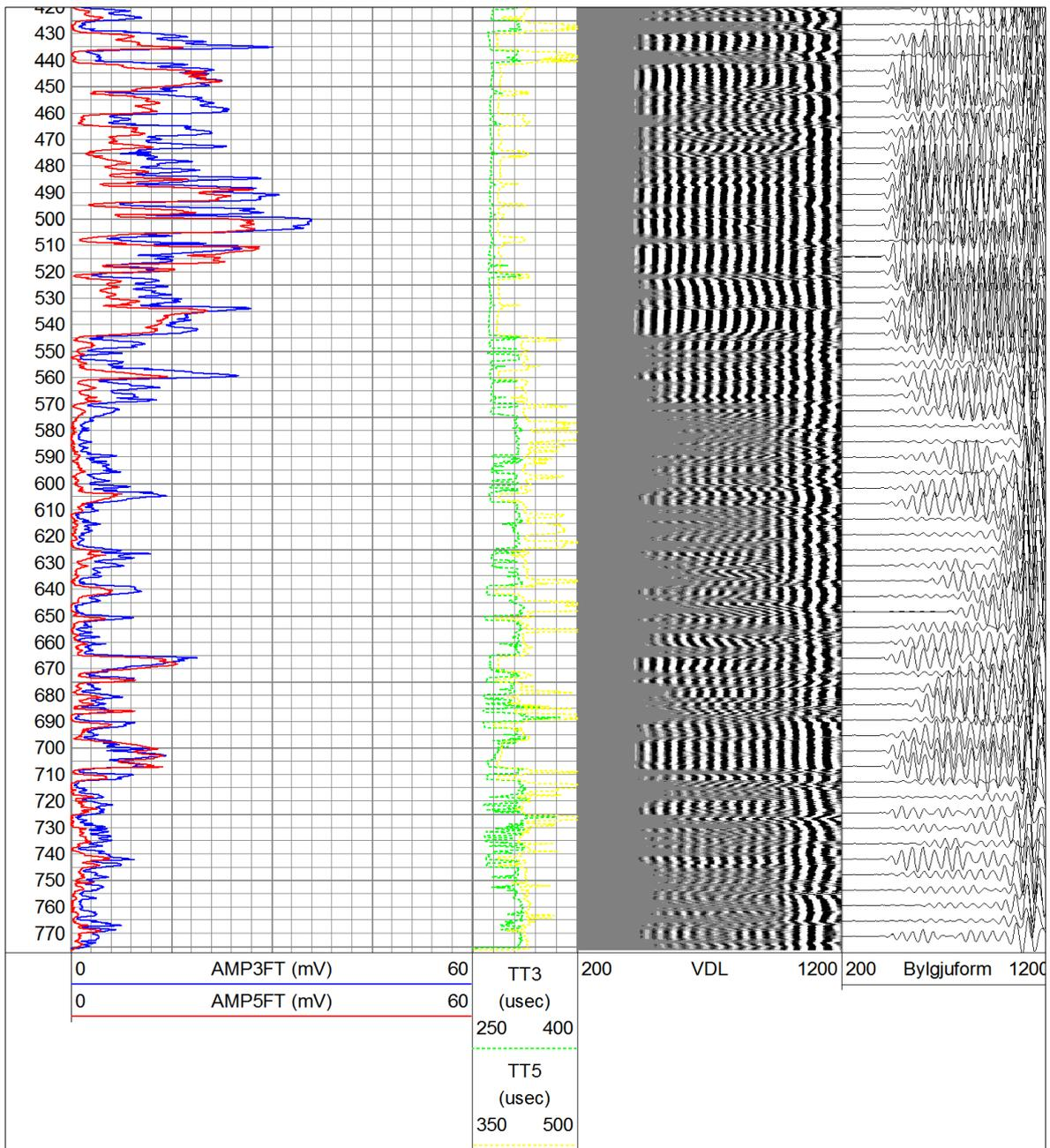
**Figure 16.** Cement Bond Log – Production casing, ~10 hours after cementing.
