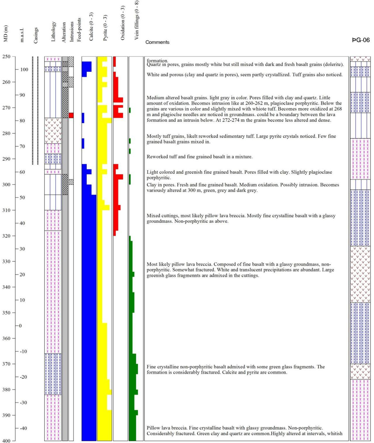
Figure 1. Lithology column from ÞG-12 from 250-400 m depth. Well ÞG-06 is shown for comparison.
