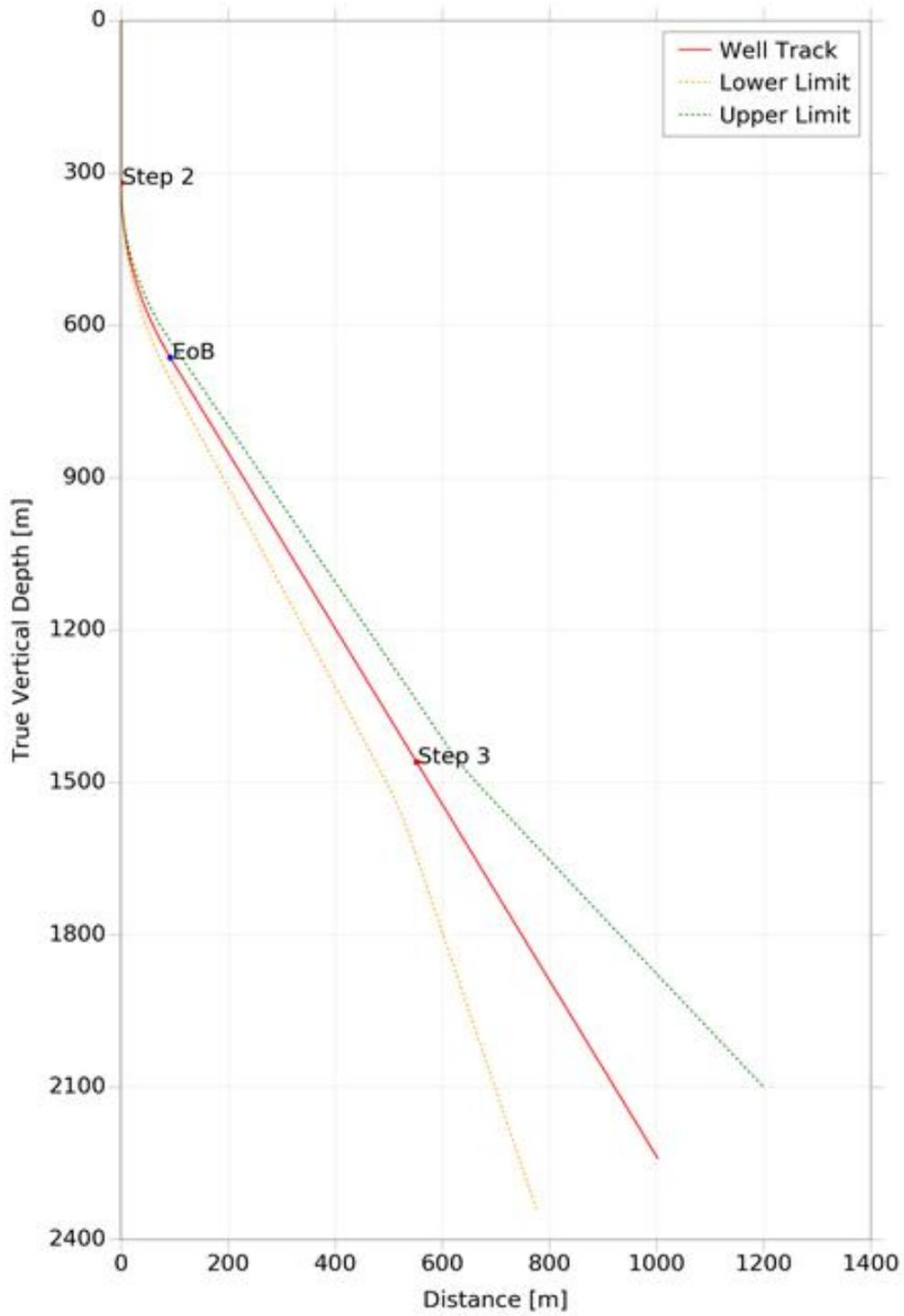
**Figure 4.** Cross section of the planned trajectory of well PG-12 with allowable deviation indicated.
