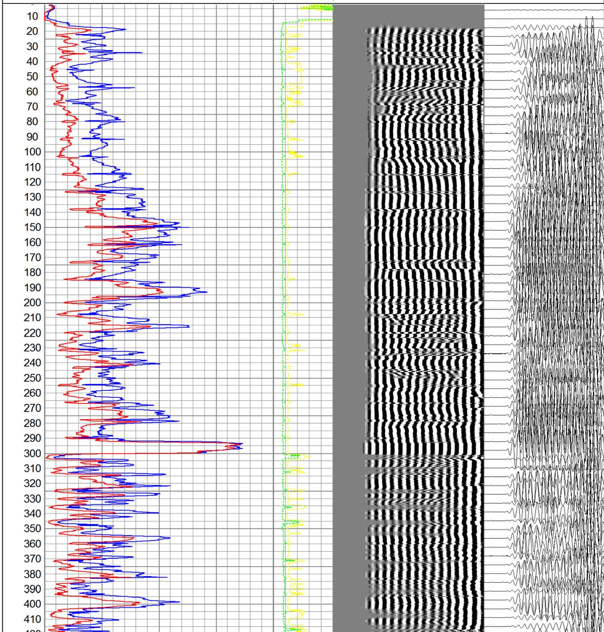
Figure 15. Cement Bond Log – Production casing, ~10 hours after cementing.
