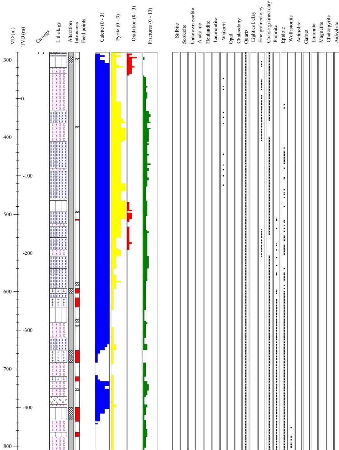
Figure 10. A summary of the alteration minerals found in ÞG-12 during drilling of phase 2.
