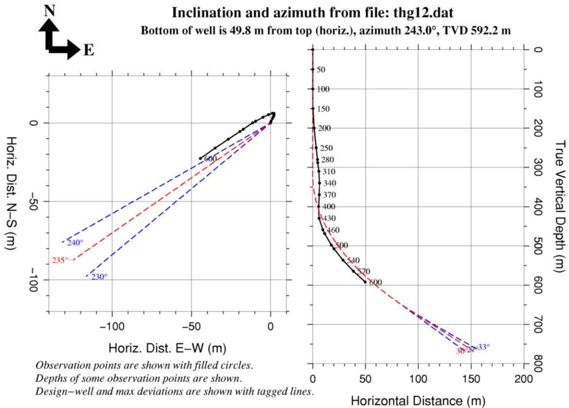
**Figure 12.** Calculated well path from the measured inclination and azimuth data together with the designed well path and corresponding deviation limits.
