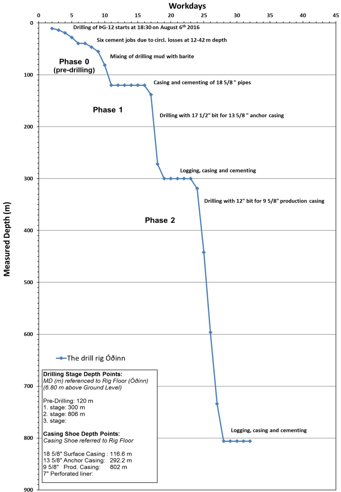
Figure 5. Drilling progress of well PG-12, phases 0–2.
