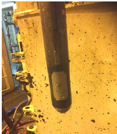
**Figure 1.** The temperature logging tool at surface after use, with the heat sensor covered by mud.
