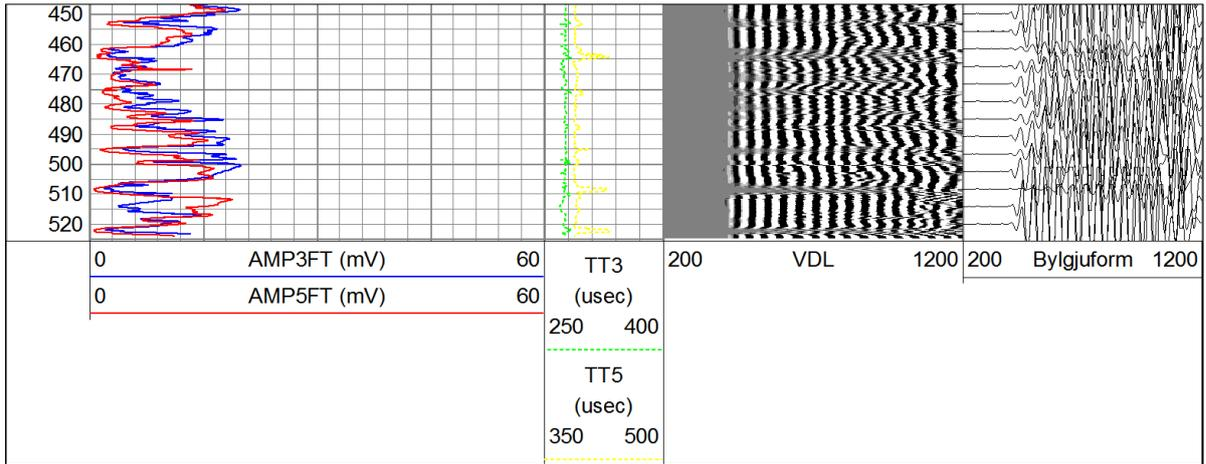
**Figure 18.** Cement Bond Log – Production casing, ~18 hours after cementing.
