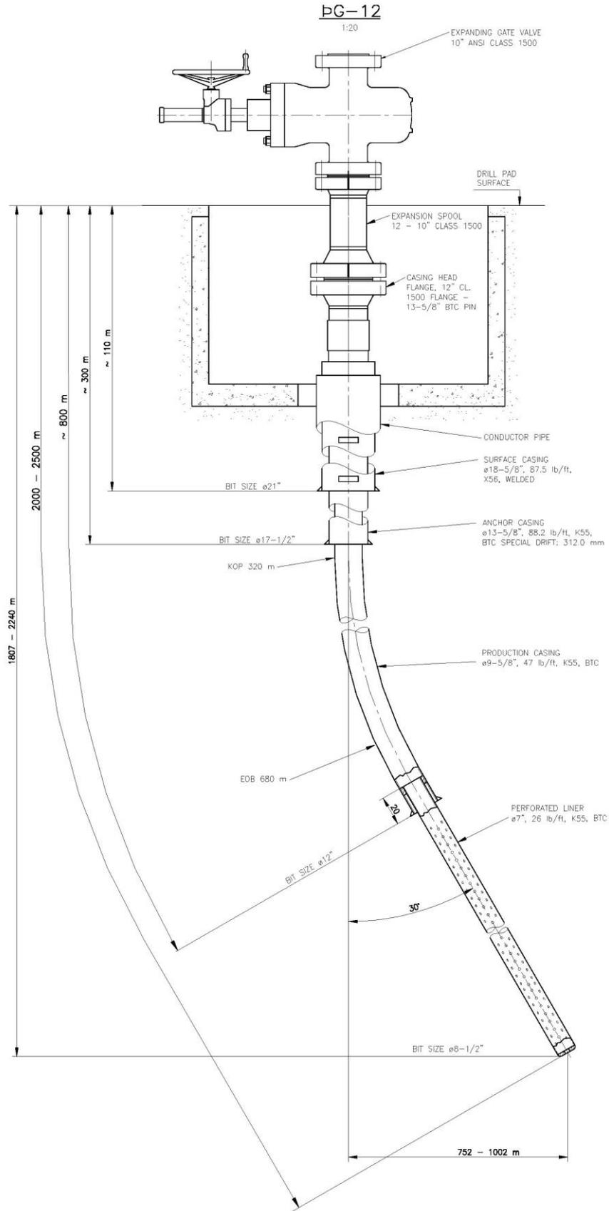
**Figure 3.** Well design of PG-12.
