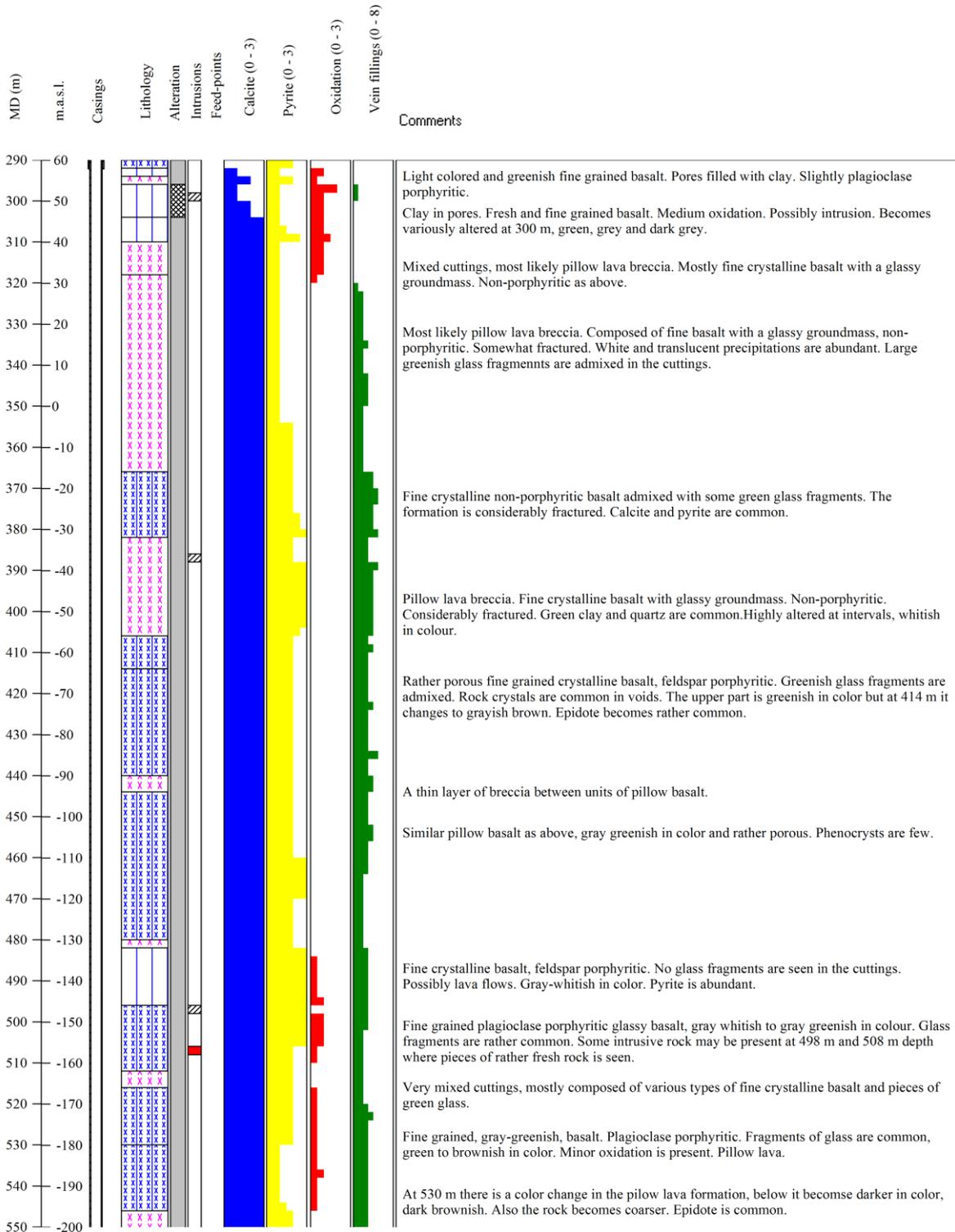
**Figure 7.** Lithology and alteration of ÞG-12, from surface to 806 m.
