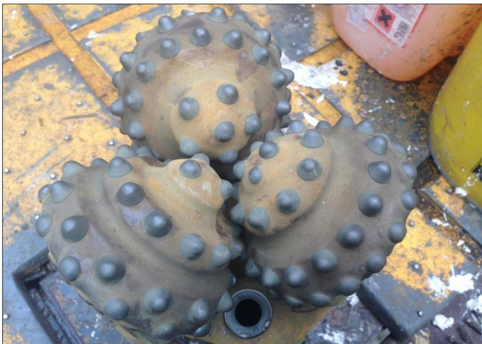
**Figure 6.** *8½" drill bit pulled out of the well on July 12<sup>th</sup>.*
