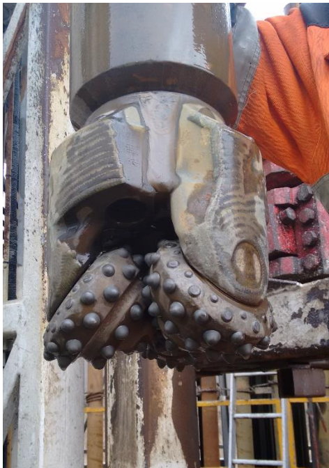
Figure 1. Drill-bit back on the surface late yesterday afternoon. The bit looks pretty good with only modest signs of wear.
