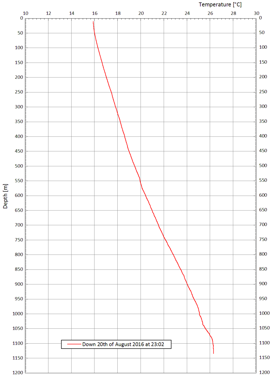
Figure 1. Temperature log RIH during 19 L/s injection and total LOC. The probe stopped at 1135 m indicating ~ 7 m bottom fill. All injected fluid seems to exit the well somewhere below 1135 m.
