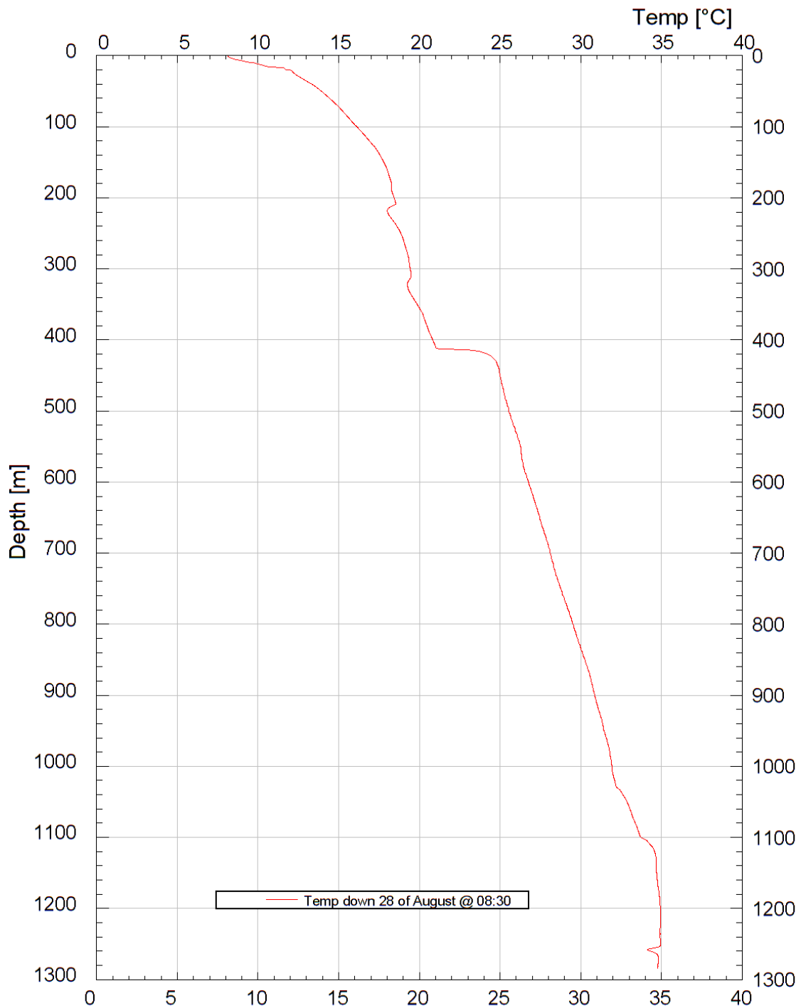
Figure 2. Temperature log inside drill-string this morning carried out prior to running in with the gyro tool. The bit is at 1302 m (MD), the tool logged down to 1285 m. Q = 19 L/s on kill line no pumping on string. Note cooling points: i) at end of casing ~1030 m (change of well diameter at 1040 m); ii) at ~1100 m; and iii) at 1260 m. Note also that the well is receiving water below ~1260 m (MD).
