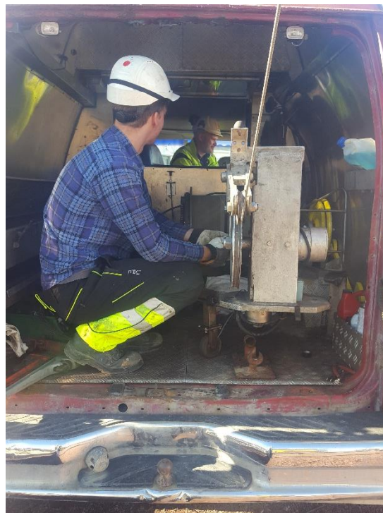
Figure 2. ÍSOR's logging engineers on site, logging temperature.
