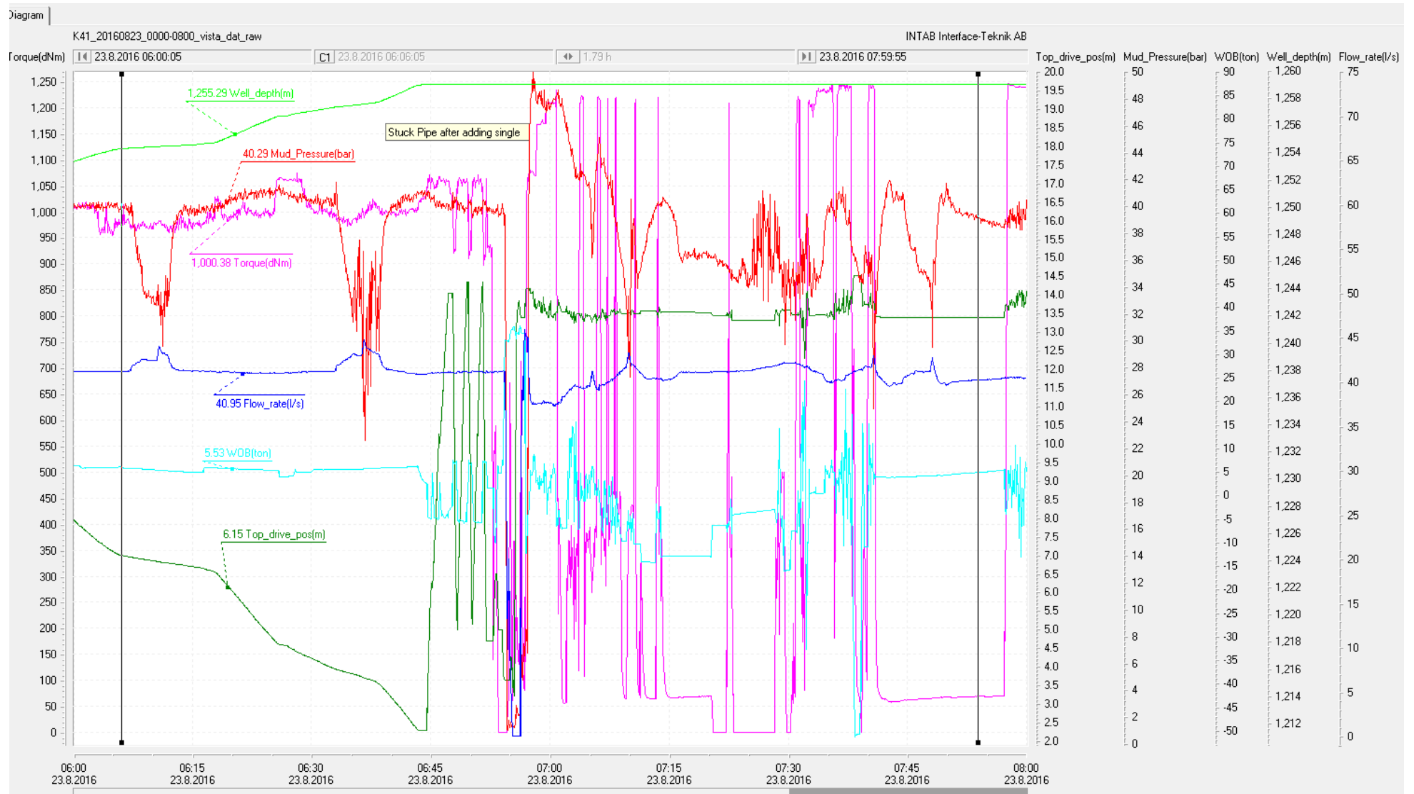
Figure 3. Key parameters during this morning's "stuck-pipe" event.
