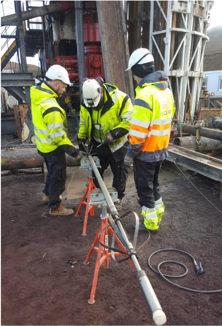
Figure 2. Picture of the ISOR logging engineers preparing the Acoustic Tele-viewer tool
