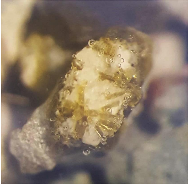
Figure 2. Calcite found over epidote at 996 m. The bubbles form when hydrochloric acid is added to the sample and CO 2 is released.
