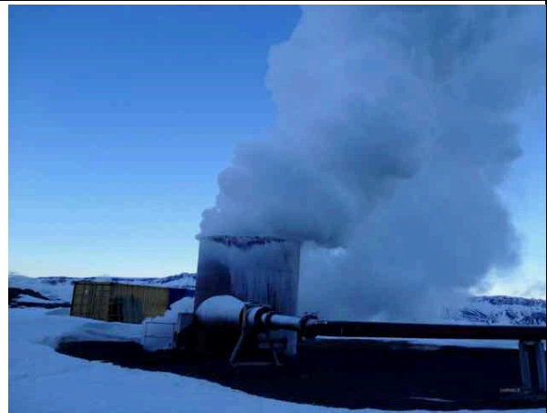
Photo 46: Well test with steam rising through silencer
