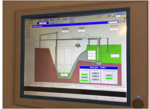
Photo 58: Ufsarlón intake gate closed for full river flow
