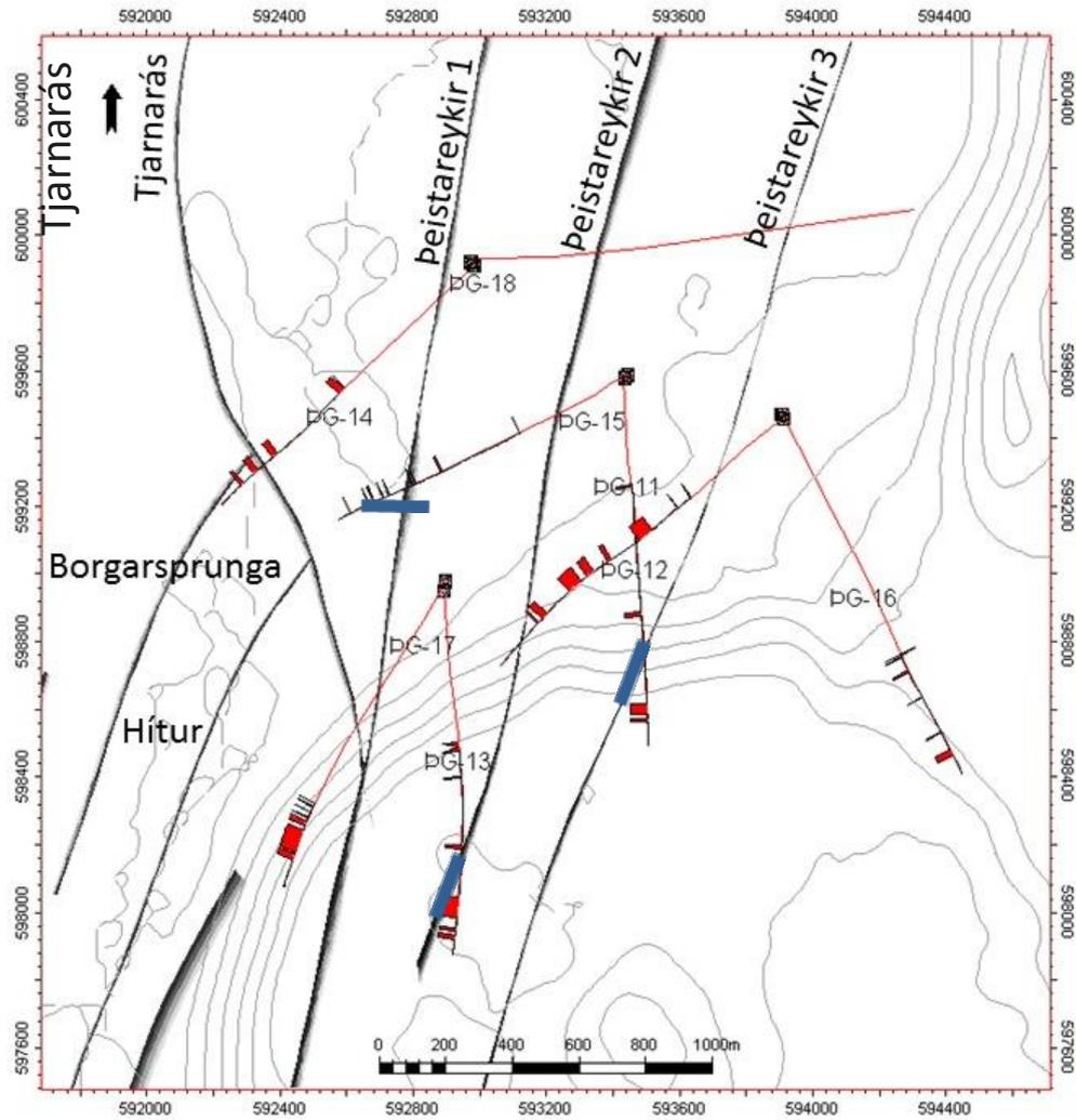
**Figure 5.** The seven faults that are included in the geological model of Beistareykir. Red intervals along the well pads show active feed zones based on spinner logging, and blue lines show the strike of faults (based on televiwer logging) in DG-11, DG-13 and DG-15, at the depths where the faults intersect the wells.
