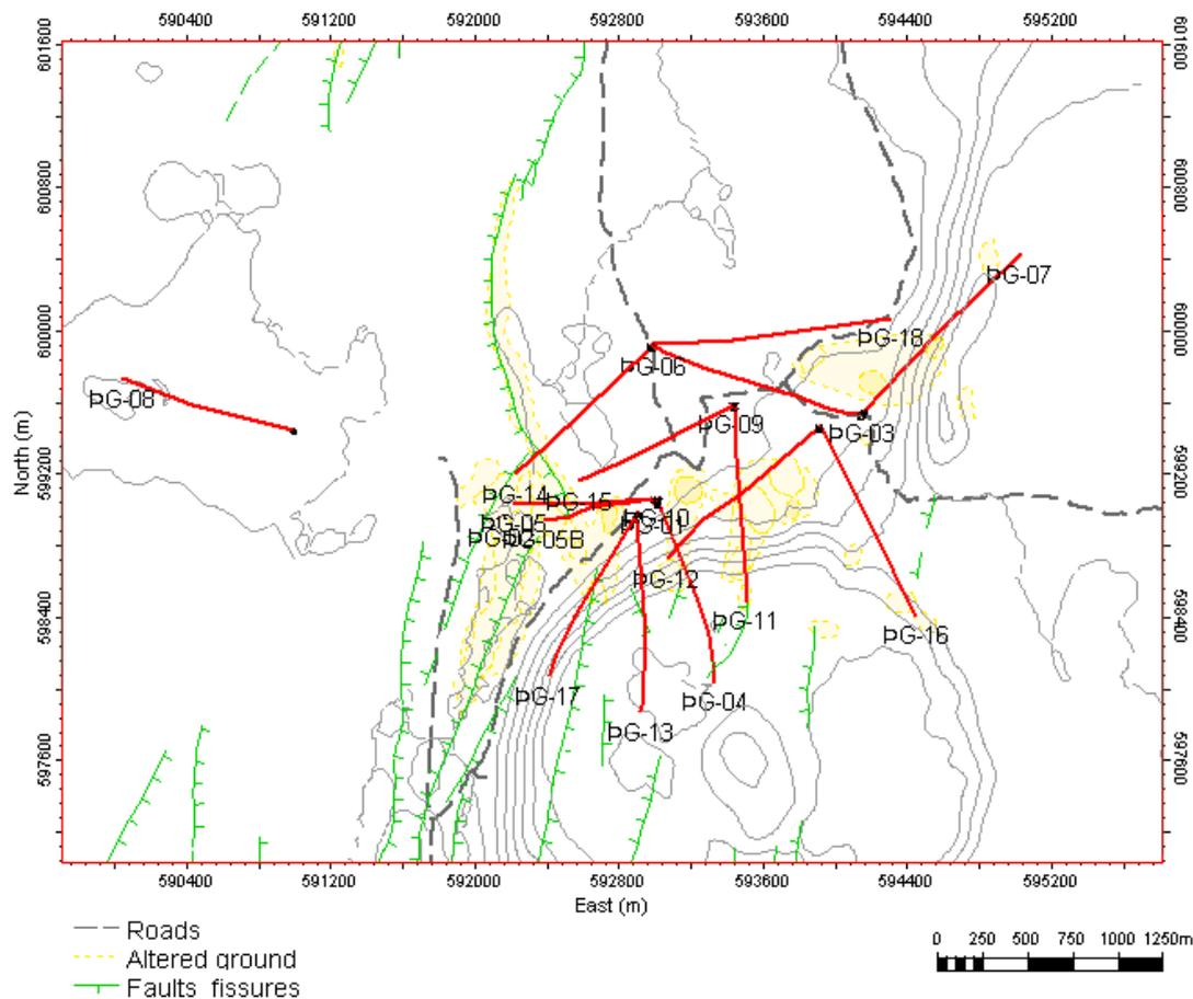
**Figure 1.** Location of the Peistareykir production wells, surface manifestations, surface faults and fissures and roads in the area.
