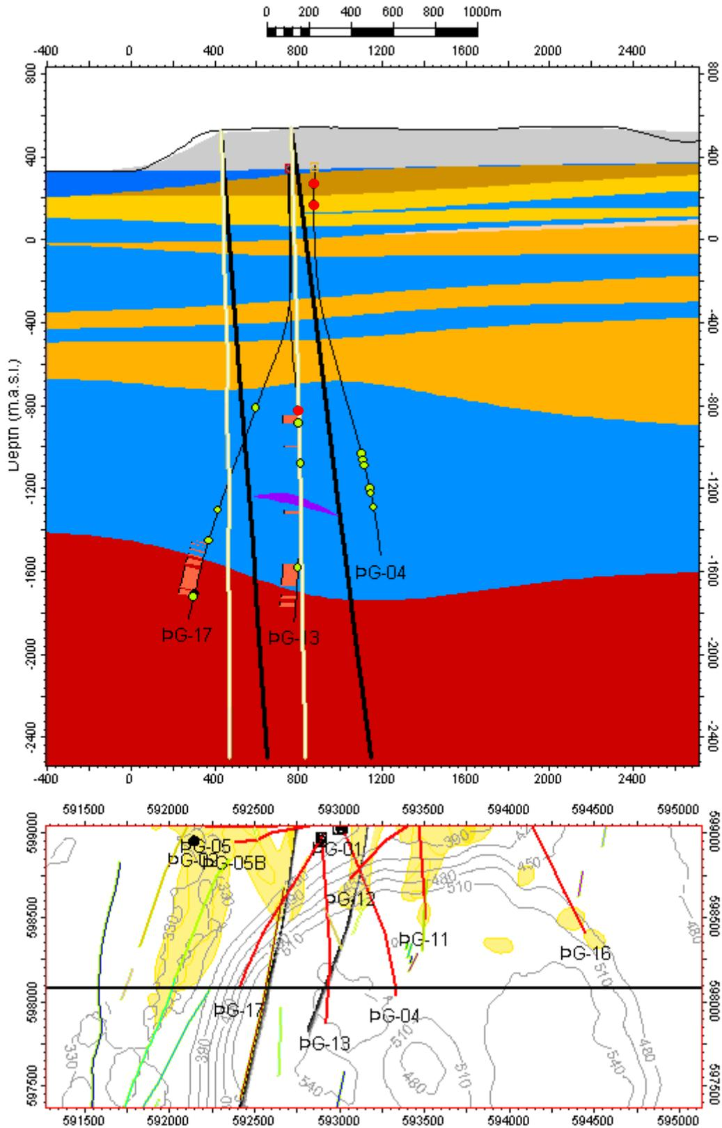
**Figure 6.** The geological model and the previous dip of two fractures in the geological model (black line). The yellow lines represent the revised dip, based on locations of medium feed zones (green dots), large feed zones (red dots), televiwer data and active feed zone (red intervals) (see color legend for geological units in Figure 3).
