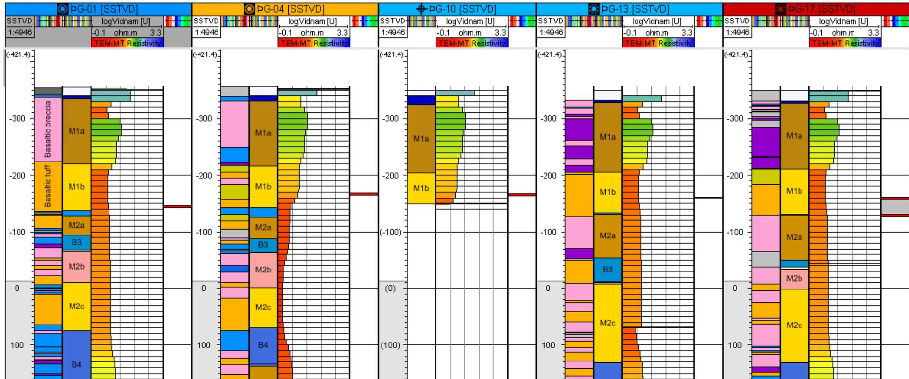
**Figure 13.** A well log section showing lithological units of the geological model (to the left), cutting analysis from the wells (in the middle) and a resistivity log, based on a 3D resistivity inversion by Karlsdóttir et al. (2012). The red intervals represent the location of the over-pressurized feed zones detected in well pad A (see color legend in Figure 3).
