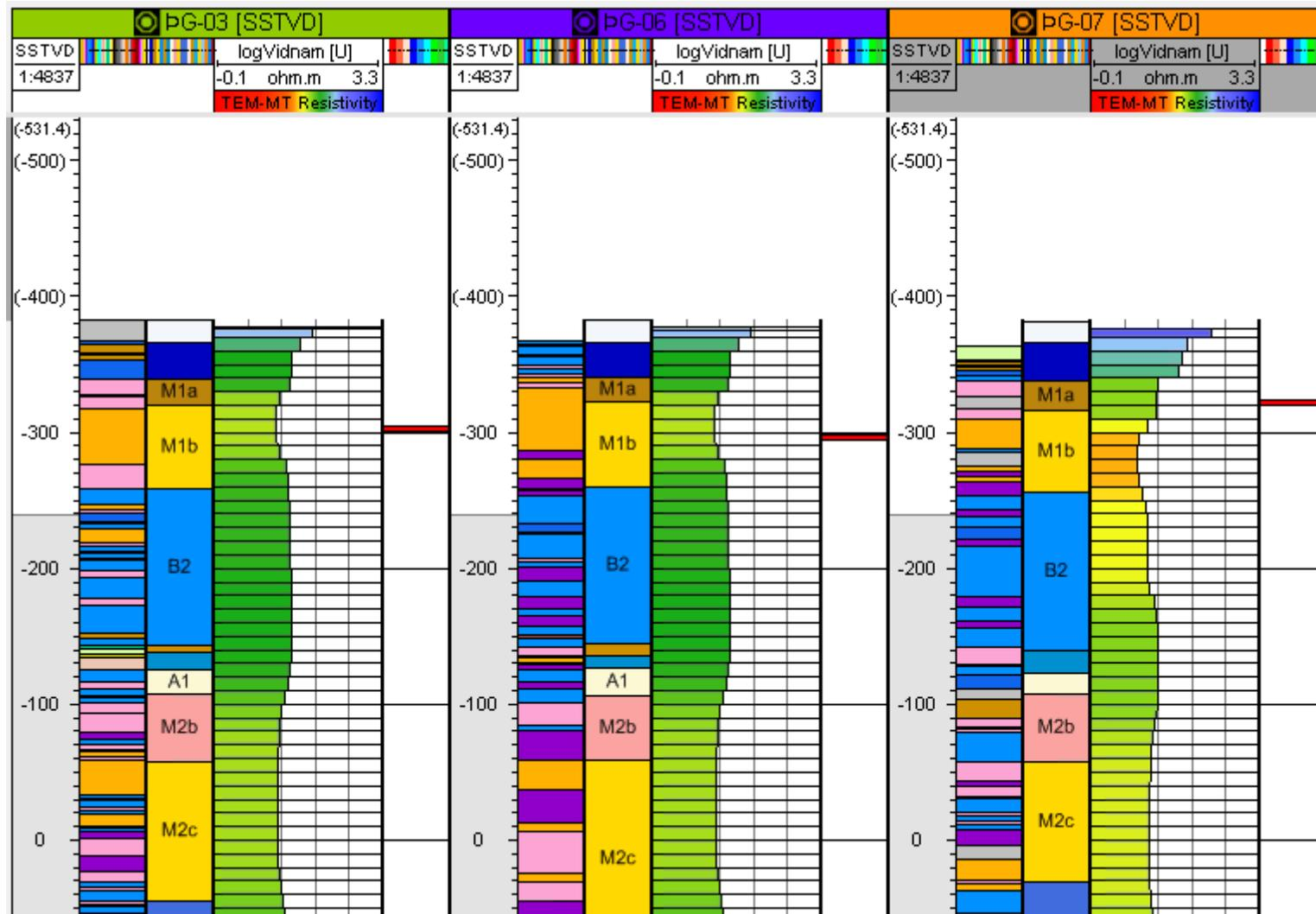
**Figure 14.** A well log section showing lithological units of the geological model (to the left), cutting analysis from the wells (in the middle) and a resistivity log, based on a 3D resistivity inversion by Karlsdóttir et al. (2012). The red intervals represent the location of the over-pressurized feed zones detected in well pad C (see color legend in Figure 3).
