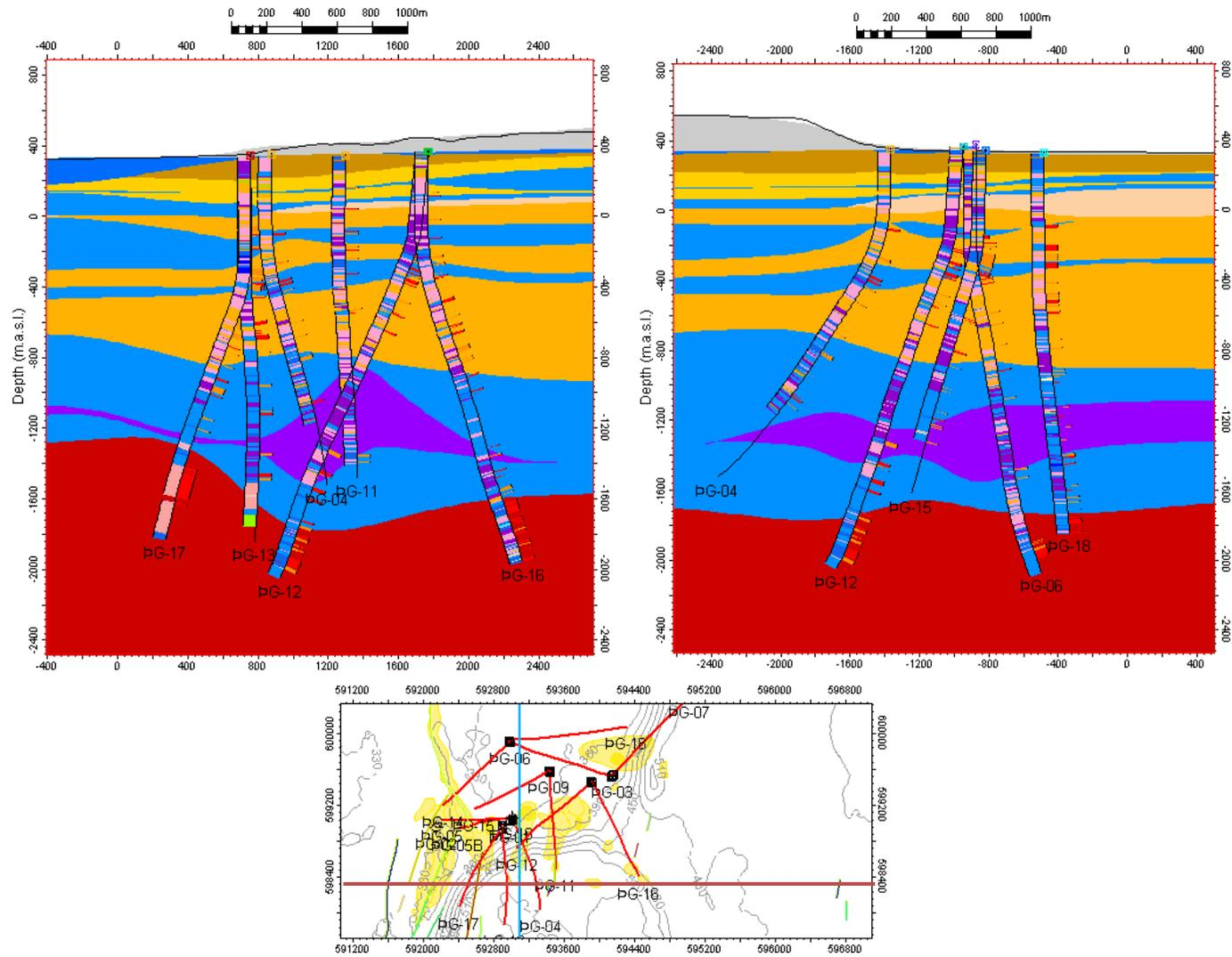
**Figure 4.** A cross section showing the units of the geological model. The left section strikes E-W (orange line on map) and the right section strikes N-S (blue line on map). Lithology logs and intrusion logs are shown on the sections (see color legend in Figure 3).
