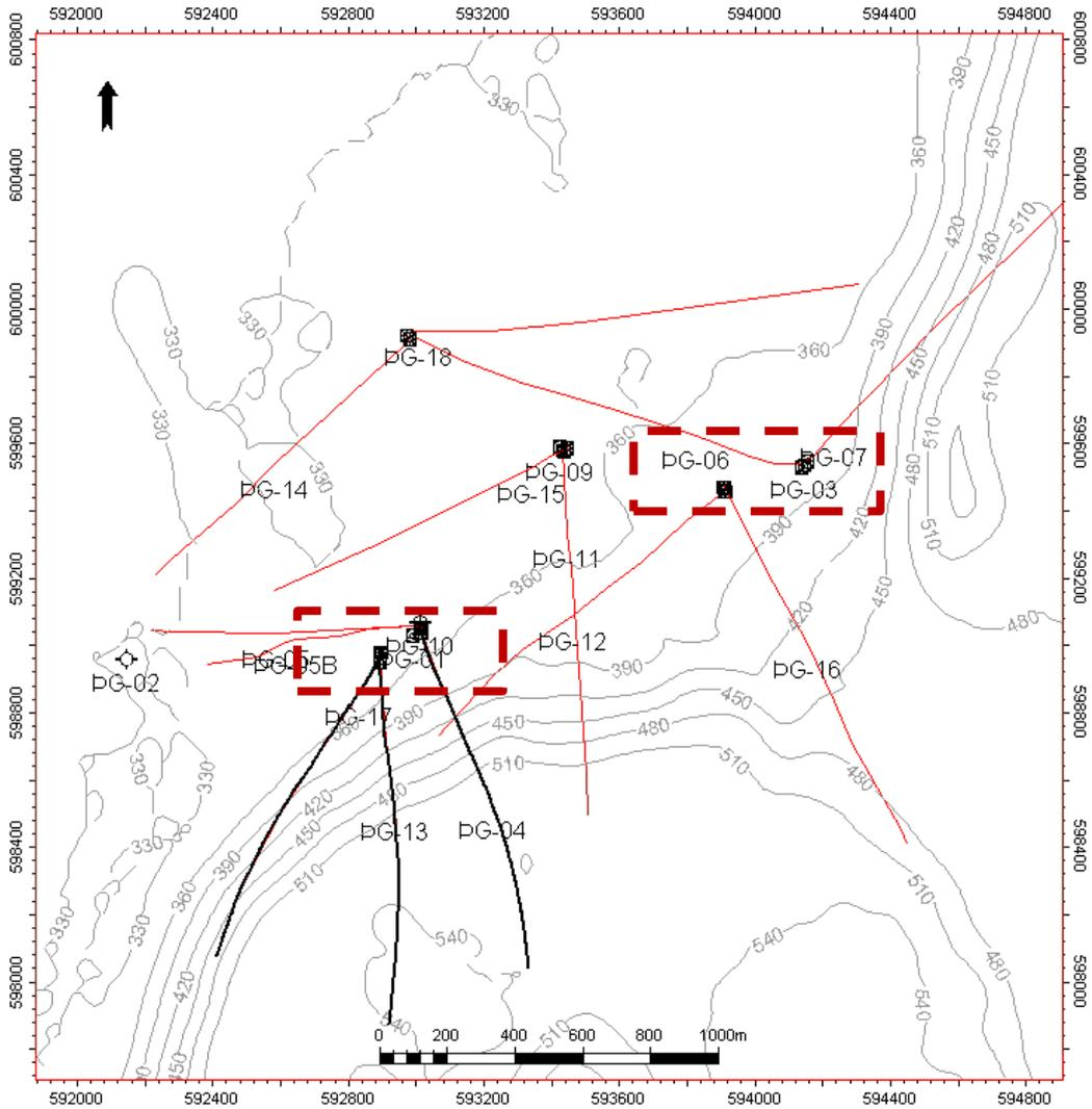
**Figure 12.** Location of well pad A and well pad C, where over-pressurized feed zones were cut. The over pressure was also recognized in well DG-9 but did not cause any problem during drilling.
