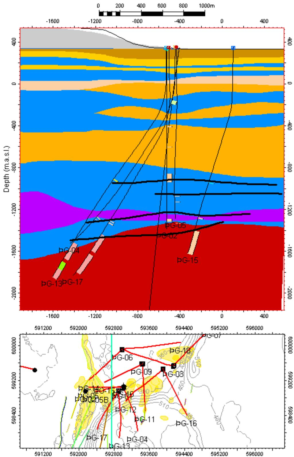
**Figure 11.** A N-S section of the geological model of Beistareykir. The interval log along well paths represents felsic or intermediate formations detected in the wells. Black lines represent the correlation between wells (see colour legend in Figure 3).
