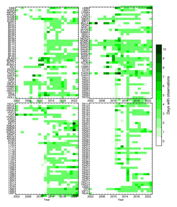
**Figure 3. Summary of campaign GNSS data available.** The color codes indicate how many days of observation each campaign site has in different years. The site names starting with TR are located in the Þeistareykir area, with first measurements in 2011.
