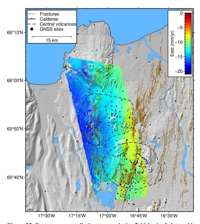
Figure 25. East-component displacement velocity field in the Þeistareykir and Krafla areas combining GNSS and InSAR observations with the SISTEM software. The InSAR displacements are derived from T111 and T147 (Figure 22 and Figure 23).
