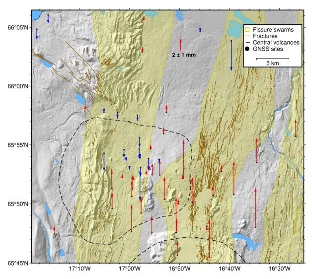
Figure 16. GNSS vertical displacement velocity field at the Peistareykir area. The light blue and light red lines indicate the uncertainties of velocity estimates (standard deviation, ~68% confidence interval).
