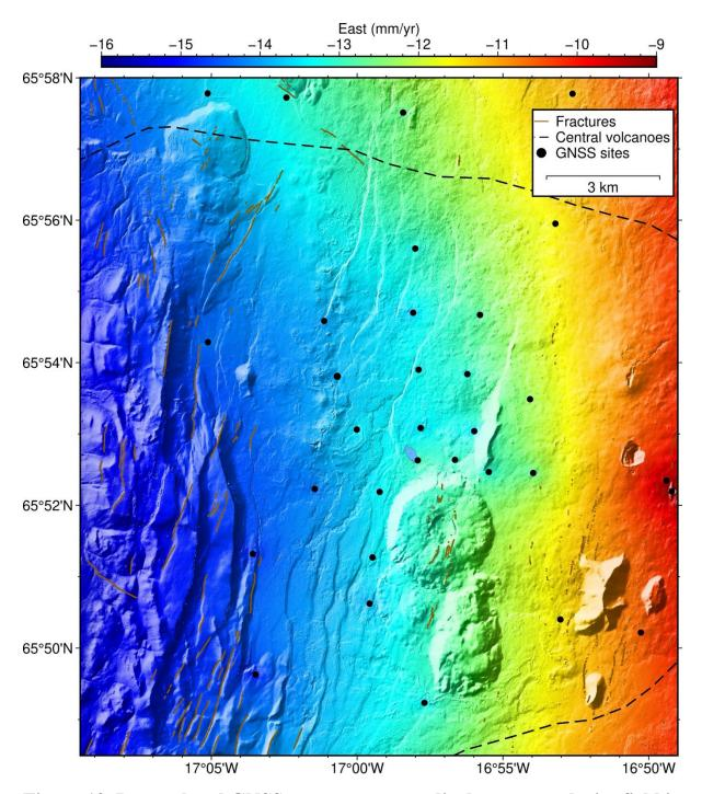
Figure 12. Interpolated GNSS east-component displacement velocity field in a smaller area of Peistareykir. The interpolation method is algorithm GPSGridder implemented in Generic Mapping Tools (GMT). See the text for the explanation of parameters.
