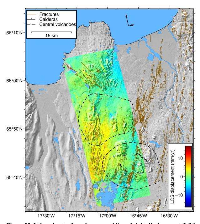
Figure 23. Inferred rate of yearly averaged line-of-sight displacement (LOS velocity) inferred from Sentinel-1 Track T147 (descending) in 2017–2022. The azimuth direction of the satellite is 347.2° to the north, and the incidence angle is 35.5°.
