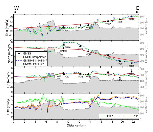
**Figure 37. Central-south profile of long-term displacement in the Peistareykir area.** The triangles show the displacement velocities at near-by GNSS sites projected onto the profile at the same longitude. GNSS interpolated, GNSS+T111+T147, and GNSS+T9+T147 are profiles extracted from corresponding maps.
