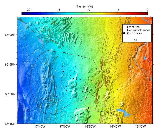
Figure 10. Interpolated GNSS east-component displacement velocity field at the Peistareykir area. The interpolation method is algorithm GPSGridder implemented in Generic Mapping Tools (GMT). See the text for the explanation of parameters.
