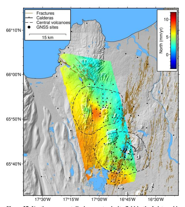
Figure 27. North-component displacement velocity field in the Þeistareykir and Krafla areas combining GNSS and InSAR observations with the SISTEM software. The InSAR displacements is derived from T111 and T147 (Figure 22 and Figure 23).
