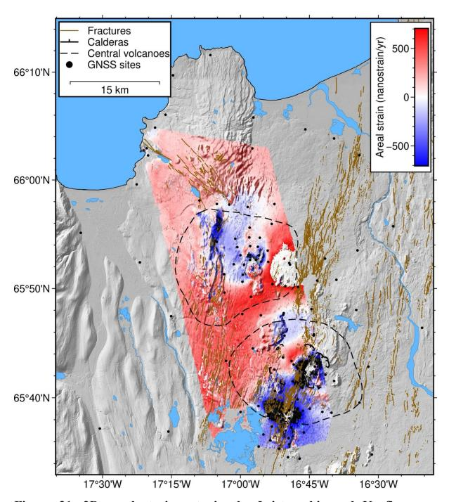
Figure 31. 2D areal strain rate in the Peistareykir and Krafla areas combining GNSS and InSAR observations with the SISTEM software. The InSAR displacements is derived from T111 and T147 (Figure 22 and Figure 23).
