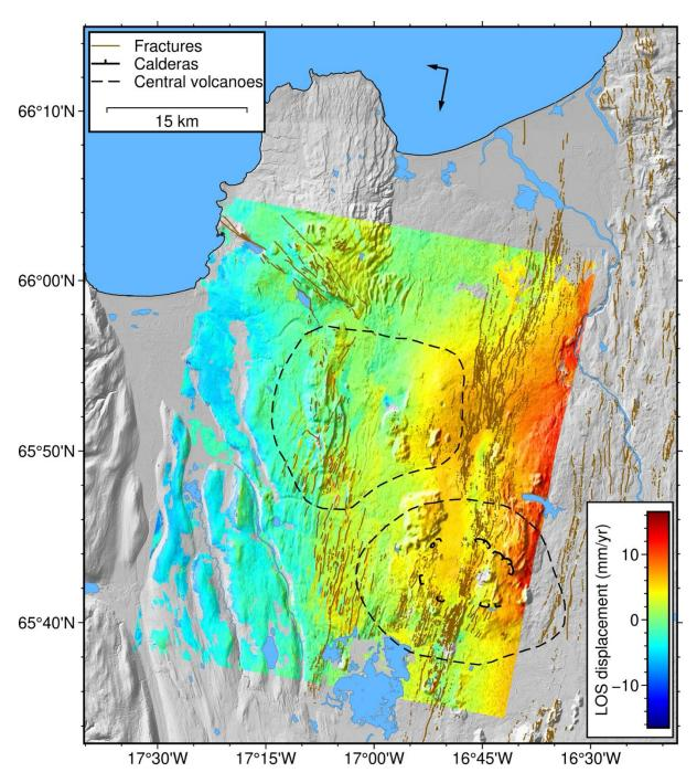
Figure 22. Inferred rate of yearly averaged line-of-sight displacement (LOS velocity) inferred from Sentinel-1 Track T111 (descending) in 2017–2022. The azimuth direction of the satellite is 190.6° to the north, and the incidence angle is 42°.
