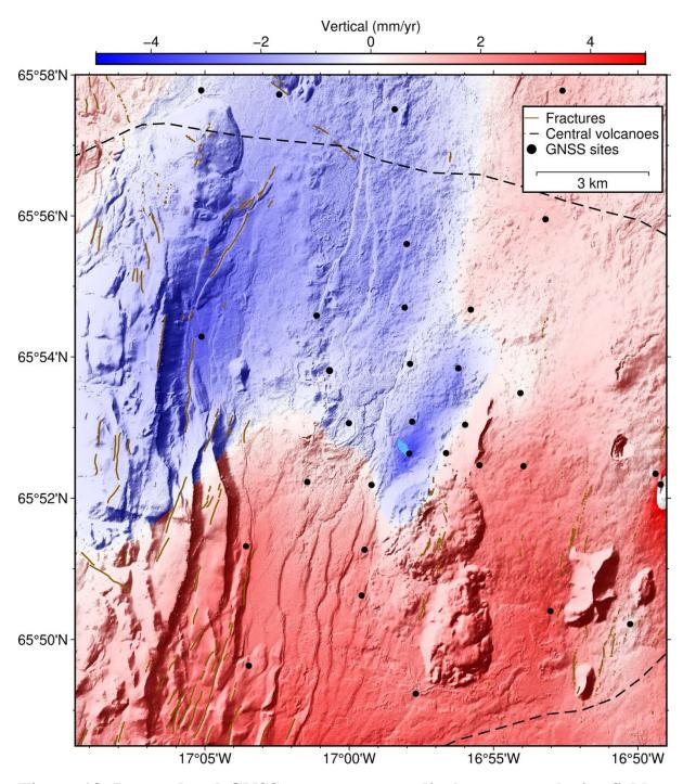
Figure 18. Interpolated GNSS up-component displacement velocity field at a smaller area of Þeistareykir. See the text for explanation of the interpolation method.
