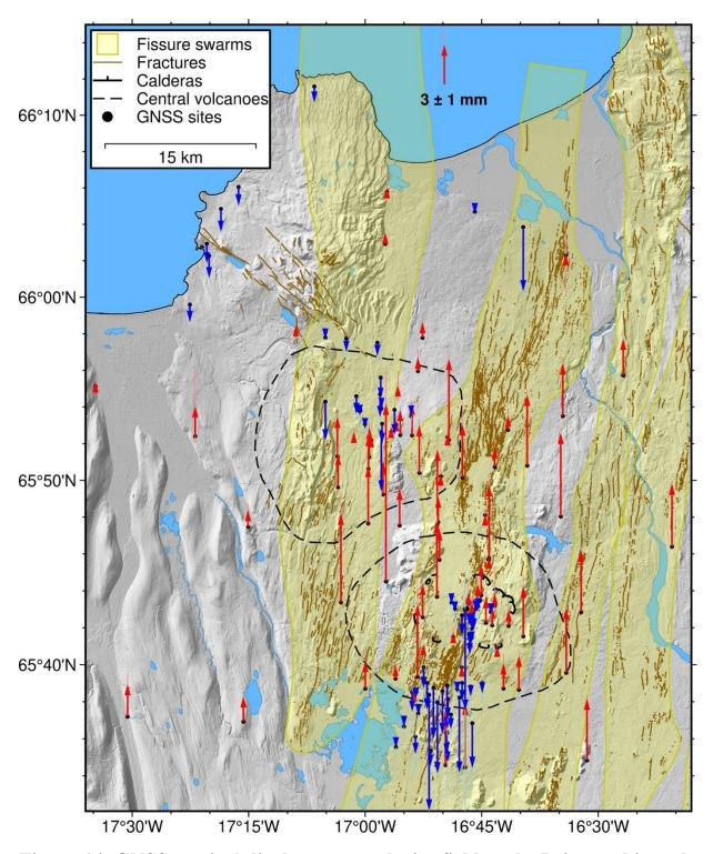
Figure 14. GNSS vertical displacement velocity field at the Peistareykir and Krafla areas. The light blue and light red lines indicate the uncertainties of velocity estimates (standard deviation,  $\sim 68\%$  confidence interval). The time span of GNSS time series deriving the velocity field is explained in the text.
