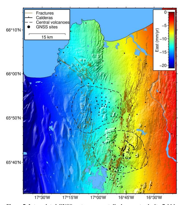
Figure 7. Interpolated GNSS east-component displacement velocity field in the Peistareykir and Krafla areas. The interpolation method is algorithm GPSGridder implemented in Generic Mapping Tools (GMT). See the text for the explanation of parameters.
