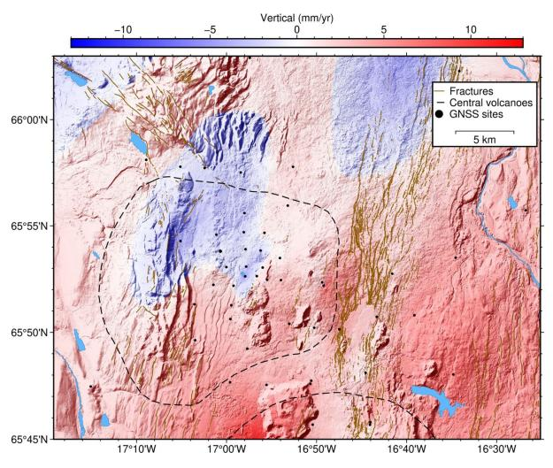
Figure 17. Interpolated GNSS up-component displacement velocity field at the Peistareykir area. See the text for explanation of the interpolation method.
