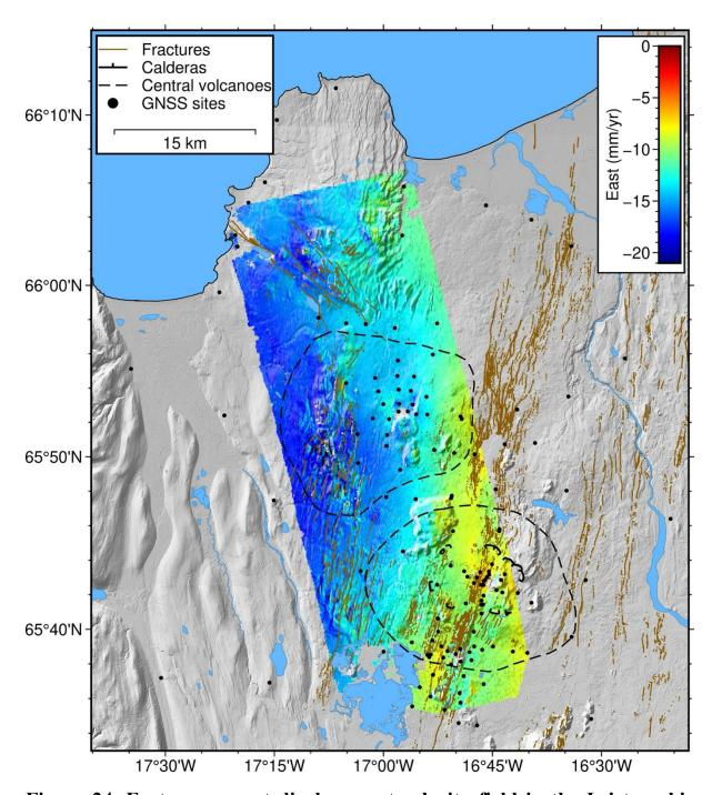
Figure 24. East-component displacement velocity field in the Peistareykir and Krafla areas combining GNSS and InSAR observations with the SISTEM software. The InSAR displacements are derived from T9 and T147 (Figure 21 and Figure 23).
