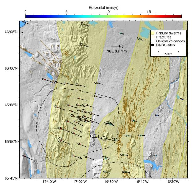
Figure 9. GNSS horizontal displacement velocity field at the Peistareykir area. The velocities are referred to Eurasian plate based on the ITRF2014 plate motion model (Altamimi et al., 2017). The ellipsoids indicate the uncertainties of velocity estimates (standard deviation, ~68% confidence interval). The arrows are color-coded according to the magnitude of horizontal velocities. The time span of GNSS time series deriving the velocity field is explained in the text.
