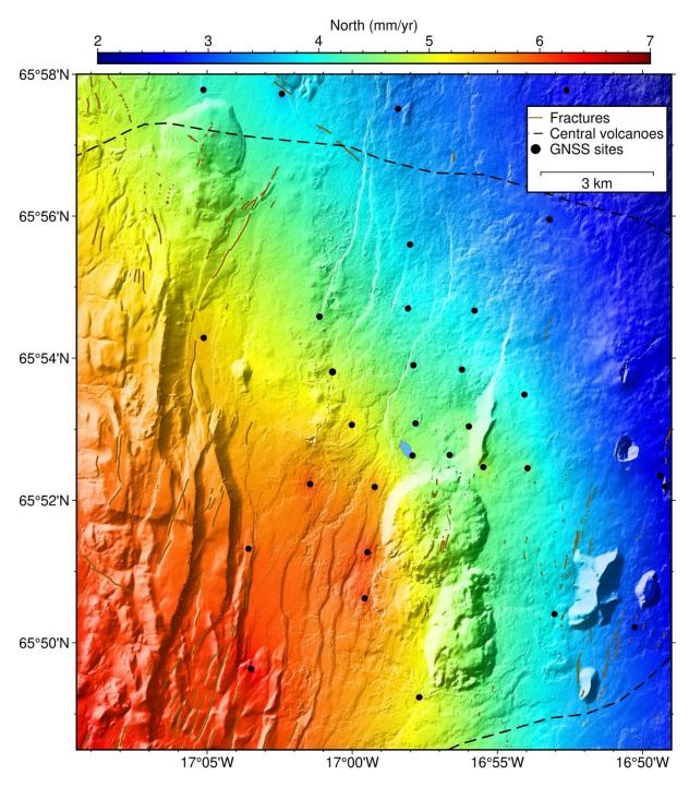
Figure 13. Interpolated GNSS north-component displacement velocity field in a smaller area of Peistareykir. The interpolation method is algorithm GPSGridder implemented in Generic Mapping Tools (GMT). See the text for the explanation of parameters.
