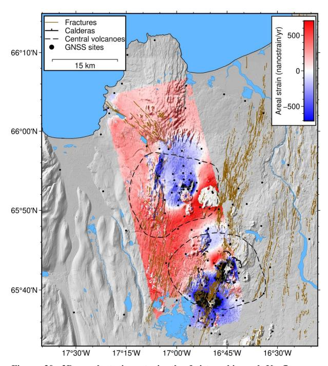
Figure 30. 2D areal strain rate in the Peistareykir and Krafla areas combining GNSS and InSAR observations with the SISTEM software. The InSAR displacements is derived from T9 and T147 (Figure 21 and Figure 23).
