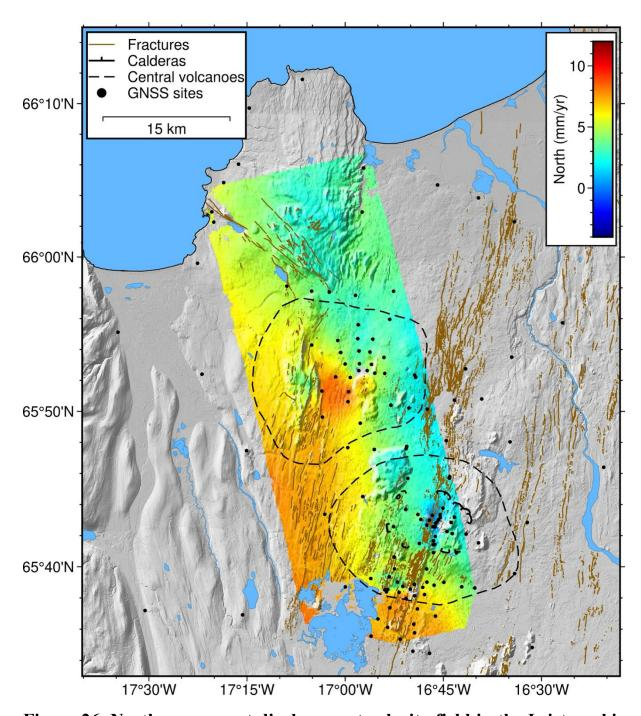
Figure 26. North-component displacement velocity field in the Þeistareykir and Krafla areas combining GNSS and InSAR observations with the SISTEM software. The InSAR displacements is derived from T9 and T147 (Figure 21 and Figure 23).
