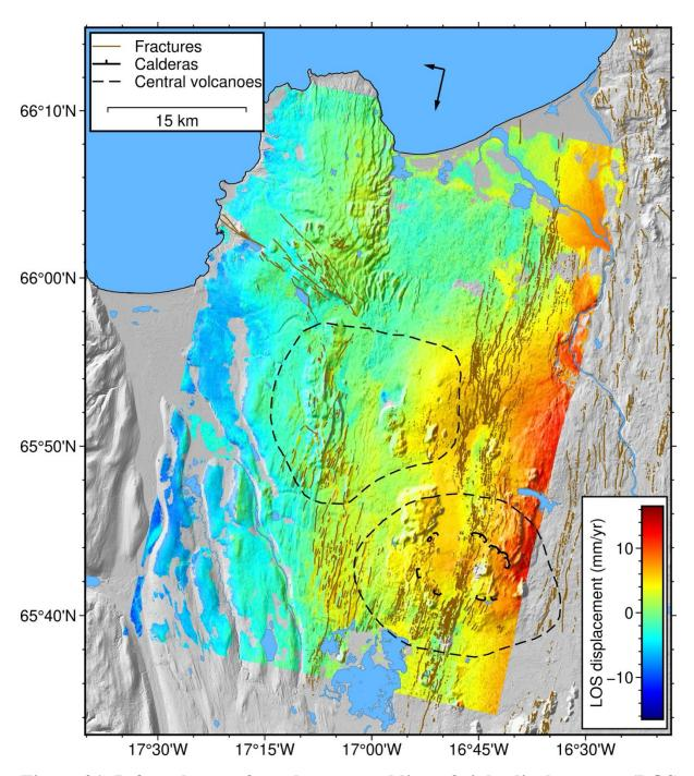
Figure 21. Inferred rate of yearly averaged line-of-sight displacement (LOS velocity) inferred from Sentinel-1 Track T9 (descending) in 2017–2022. The azimuth direction of the satellite is 192.5° to the north, and the incidence angle is 36.6°.
