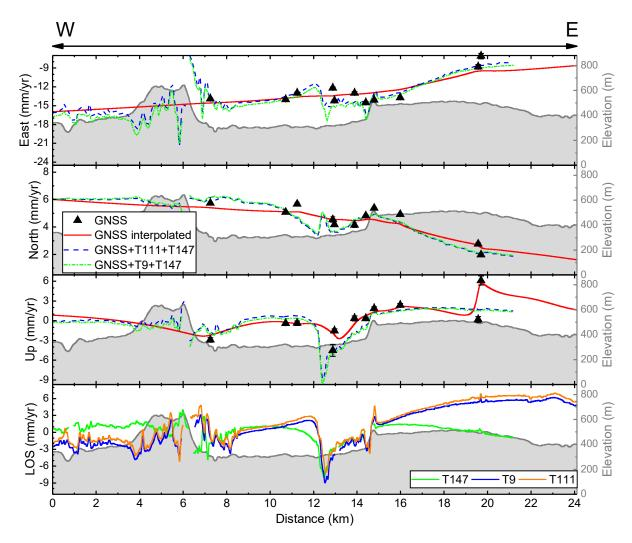
**Figure 38.** Central-north profile of long-term displacement in the **Peistareykir area.** The triangles show the displacement velocities at near-by GNSS sites projected onto the profile at the same longitude. GNSS interpolated, GNSS+T111+T147, and GNSS+T9+T147 are profiles extracted from corresponding maps. The GNSS site names from west to south are TR04, THRC, TR44, TRG1, THER, TRG2, TR12, TR24, BOND, SANF, and TR26.
