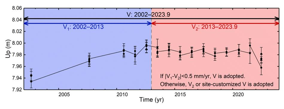
**Figure 5. Illustration of GNSS time series analysis strategy for displacement velocity estimation.** The exemplified time series is the up component at site RAUH. V represents displacement velocity.
